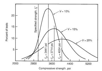
Fig. 3-4 Normal frequency curves for coefficients of variation of 10, 15, and 20 percent. (From [3-10].)
