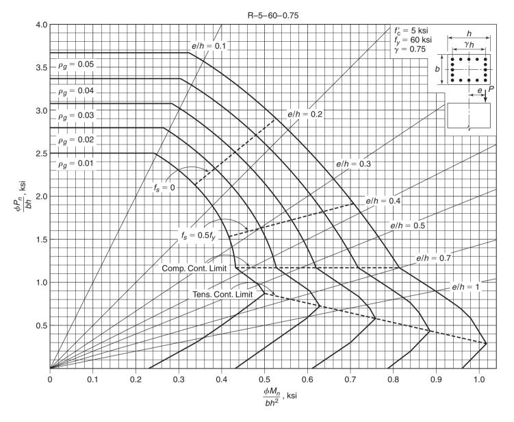
Fig. A-10b Nondimensional interaction diagram for tied column with bars in four faces:  $f'_c = 5000$  psi and  $\gamma = 0.75$ .
