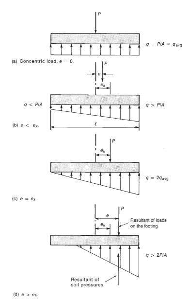
Fig. 15-5 Pressures under an eccentrically loaded footing.
