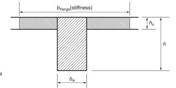
Fig. 5-16 Effective beam section for flexural stiffness analysis of a floor beam carrying gravity loading.
