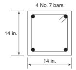
Fig. 12-29 Final column section for Example 12-2.
