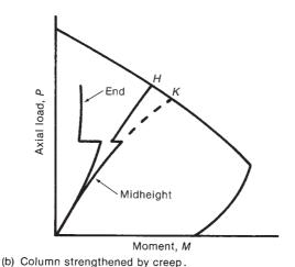
Fig. 12-23 Effect of sustained loads on moments in columns in braced frames.
