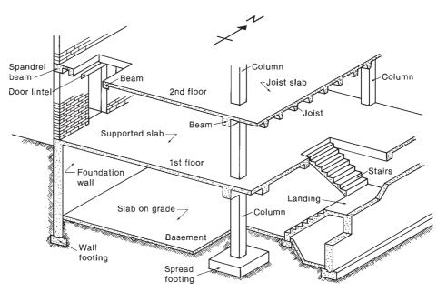
Fig. 1-6 Reinforced concrete building elements. (Adapted from [1-1].)
