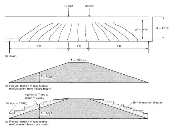
Fig. 8-20 Tension in longitudinal reinforcement.
