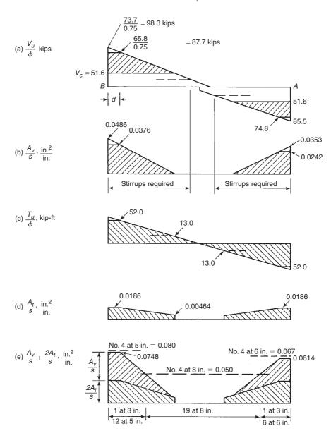
Fig. 7-35 Calculation of stirrups for shear and torsion— Example 7-4.
