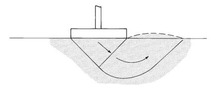
Fig. 15-3 Bearing failure of a footing.
