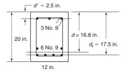
Fig. 4-35 Beam section used for Example 4-4.
