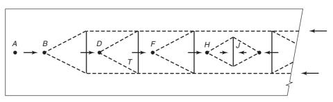
(b) Strut-and-tie model of compression flange.
