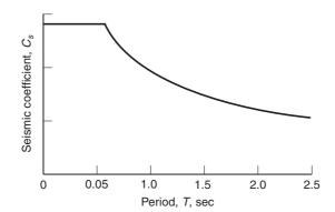
Fig. 19-11 Variation of seismic response coefficient,  $C_s$ , with period, T.
