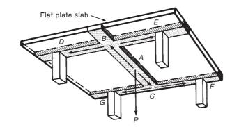
Fig. 13-1 Two-way flexure.
