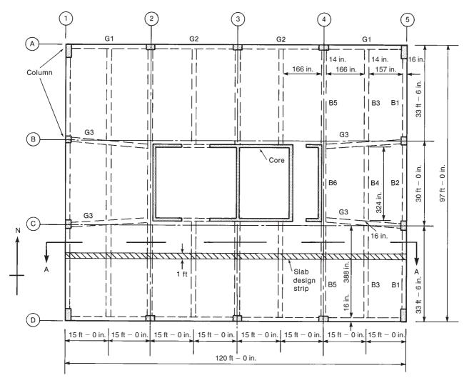
Fig. 5-34 Typical floor plan for Example 5-7.
