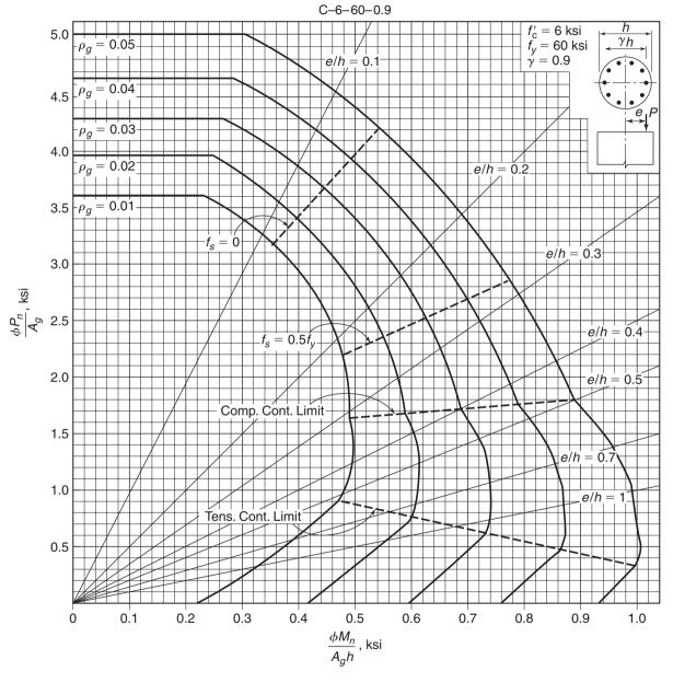
Fig. A-14c Nondimensional interaction diagram for circular spiral column:  $f'_c = 6000$  psi and  $\gamma = 0.90$ .
