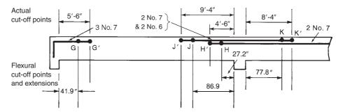
Fig. 10-10 Calculation of bar cut-off points for negative-moment steel.
