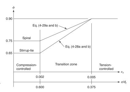
Fig. 4-24 Variation of  $\phi$ -factor with  $\varepsilon_t$  and  $c/d_t$  for spiral and stirruptie transverse reinforcement.
