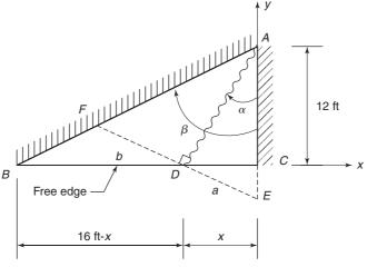
(a) Slab panel and plastic mechanism.
