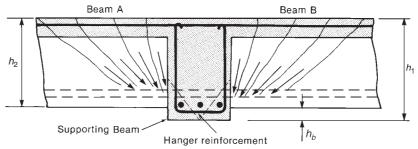
(a) Compression fan at beam-girder joint.
