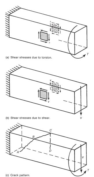
Fig. 7-9 Combined shear, torsion, and moment.
