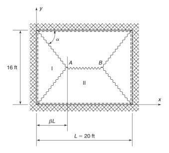
Fig. 14-10 Slab panel and plastic mechanism for Example 14-4.
