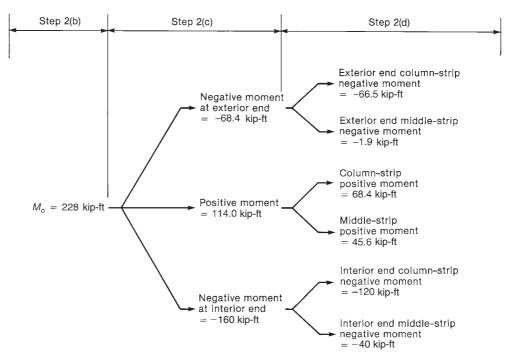
Fig. 13-29 Calculation of moments in an end span for Example 13-4.
