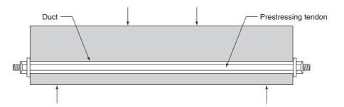
Fig. 1-5 Prestressed concrete beam.
