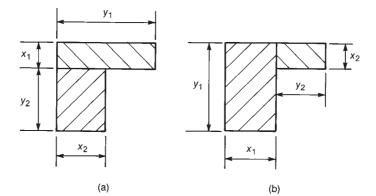
Fig. 13-24 Division of edge members for calculation of torsional constant, *C*.
