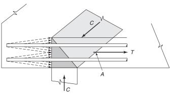
Fig. 17-10 Hydrostatic nodal zones in planar structures.
