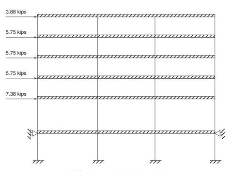
Fig. 12-33 Frame analysis model for combined gravity and lateral loading.
