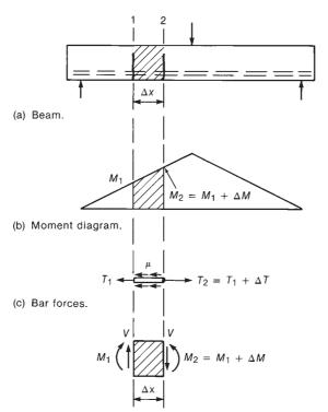
Fig. 8-3 Average flexural bond stress.
