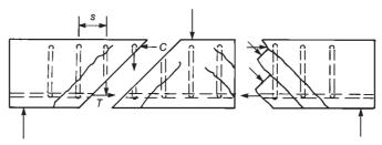
(a) Internal forces in a cracked beam.
