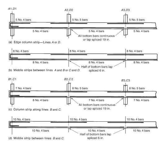
Fig. 13-90 Schematic diagram of reinforcement in north–south strips for Example 13-14.
