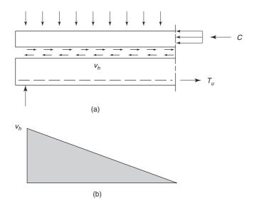
Fig. 16-12 Horizontal shear stresses in a composite beam.
