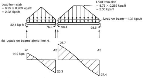
Fig. 13-99 Factored shear on edge beam for Example 13-15.
