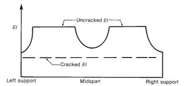
Fig. 9-12 Variation of *EI* along the length of the beam shown in Fig. 9-10b.
