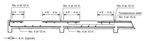
Fig. 5-37 Slab reinforcement for Example 5-7.
