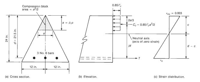
Fig. 4-20 Analysis of arbitrary cross section—Example 4-2.
