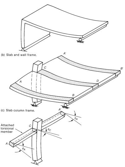
Fig. 13-38 Frame action and twisting of edge member.
