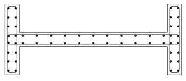
Fig. 18-16 Structural walls with concentrated reinforcement at their edges.
