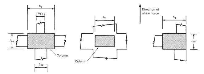
Fig. 17-55 Width of joint,  $b_i$ .
