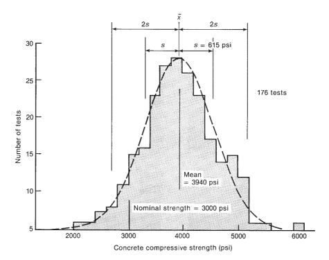
Fig. 3-3 Distribution of concrete strengths.
