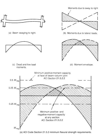
Fig. 19-17 Moment diagram due to gravity loads and seismic loads.
