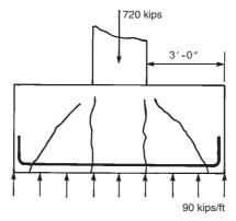
Fig. 15-23 Transverse beam at interior column—Example 15-5.
