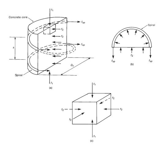
Fig. 11-4 Triaxial stresses in core of spiral column.
