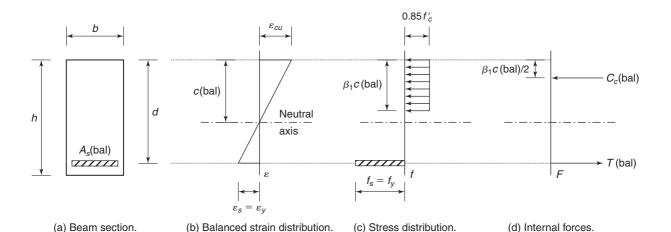
Fig. 4-21 Steps in analysis of  $A_s$ (bal), singly reinforced rectangular section.
