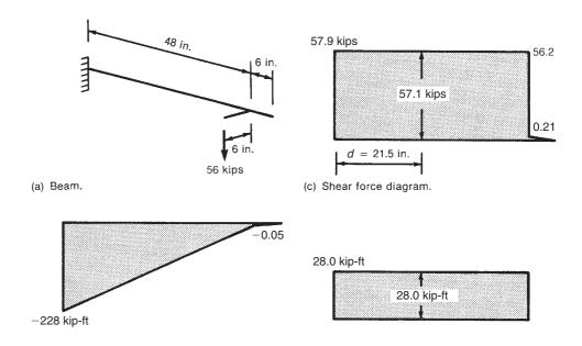
Fig. 7-28 Cantilever beam— Example 7-2.
