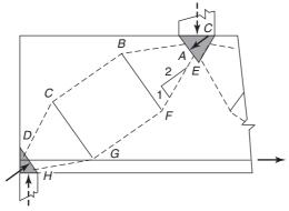
(c) Strut-and-tie model of a bottle-shaped strut.
