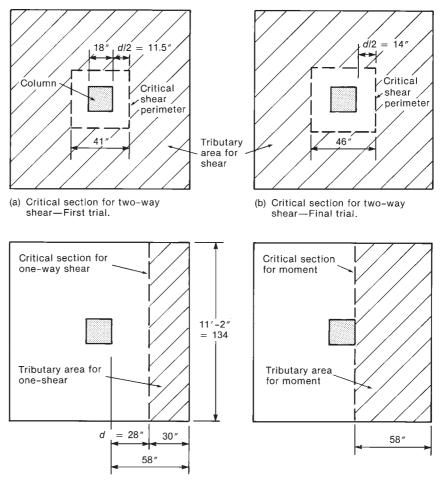
Fig. 15-14 Critical sections— Example 15-2.
