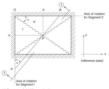
(a) Geometry of yield-line mechanism.
