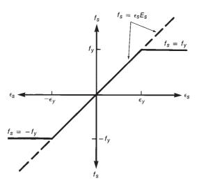
Fig. 11-15 Calculation of stress in steel from Eq. (11-11).
