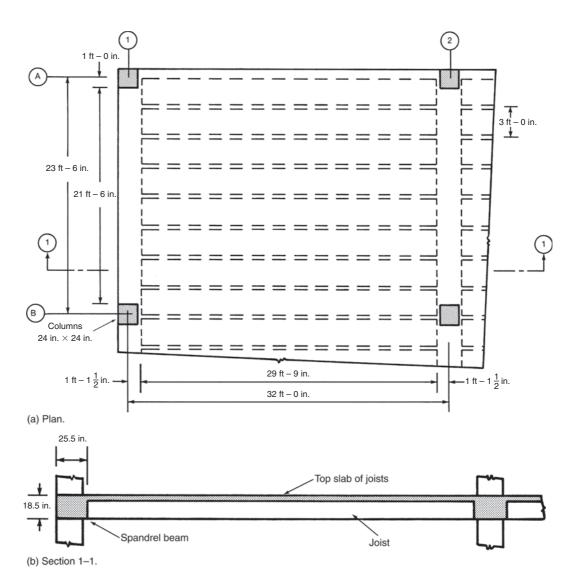
Fig. 7-30 Joist floor—Example 7-4.
