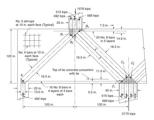
Fig. 17-37 Final design, two-span deep beam—Example 17-3.
