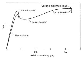
(a) Axially loaded columns.
