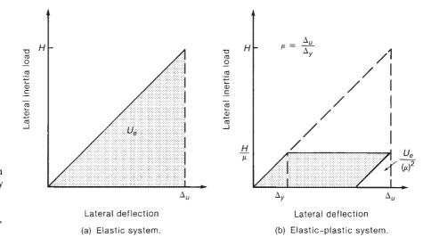
Fig. 19-4 Effect of ductility ratio,  $\mu$ , on lateral force and strain energy in structures deflected to the same  $\Delta_u$ . (From [19-12], copyright John Wiley & Sons, Inc.)
