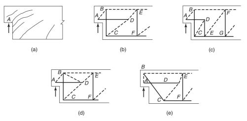
Fig. 17-42 Comparison of strut-and-tie models for dapped ends.
