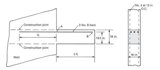
Fig. 8-16 Cantilever beam—Examples 8-1 and 8-1M.
