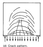
Fig. 17-28 Deep beam uniformly loaded on the bottom edge. (Adapted from [17-1].)
