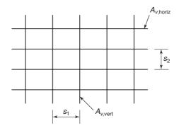
Fig. 18-20 Distribution of vertical and horizontal shear reinforcement in the web of a shear wall.
