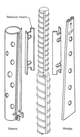
Fig. 11-27 Wedged sleeve bar splice: compression only. (Drawing courtesy of Gateway Building Products.)
