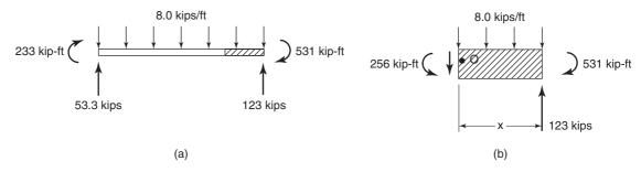
Fig. 19-24 Calculation of cutoff points—frame swaying to the right—Example 19-1.
