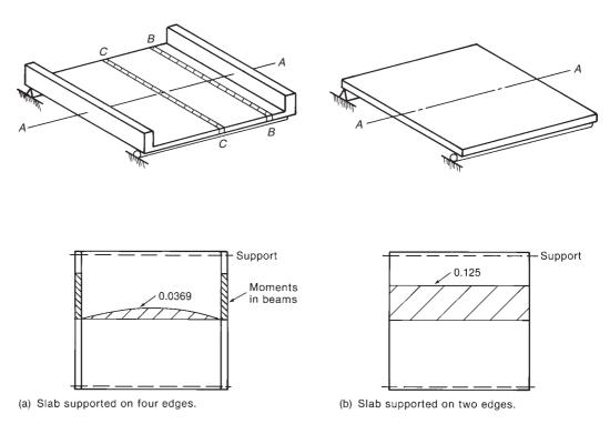
Fig. 13-13 Effect of beam stiffness on moments in slabs.
