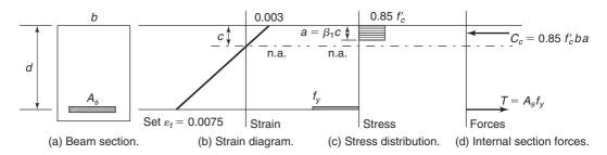
Fig. 5-27 Assumptions for design of singly reinforced beam section.
