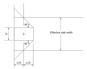
Fig. 13-48 Minimum value for effective slab width at exterior slab-to-column connections.
