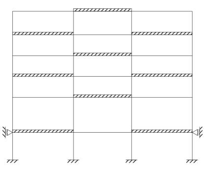
Fig. 12-34 Live-load cases considered for column moment in Example 12-3.
