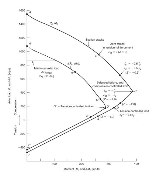
Fig. 11-18 Interaction diagram— Example 11-1.
