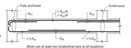
Fig. 8-27 Requirements for longitudinal structural-integrity reinforcement in perimeter beams. (*Note:* required closed transverse reinforcement not shown.)
