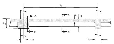
(a) Slab with beams in two directions.
