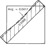
Fig. 13-12 Moments in a square slab hinged on four edges. (From [13-4].)
