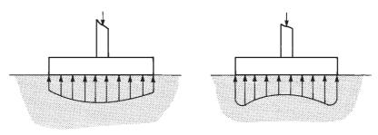
Fig. 15-2 Pressure distribution under footings.
