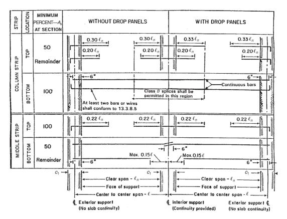
Fig. 13-83 Minimum cut-off points for slabs without beams. (From ACI Code Section 13.3.8.1.)
