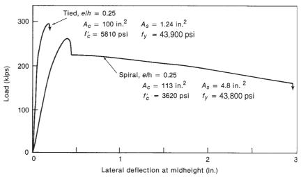
Fig. 11-5 Load-deflection behavior of tied and spiral columns. (Adapted from [11-1].)
