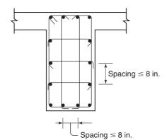
Fig. 19-36 Alternate procedure for confinement reinforcement in coupling beams.
