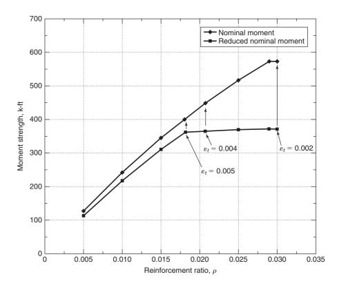
Fig. 4-26 Relationship between  $\rho$  and values for  $M_n$  and  $\phi M_n$ .
