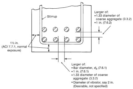
(b) Minimum bar spacing and cover limits in ACI Code.
