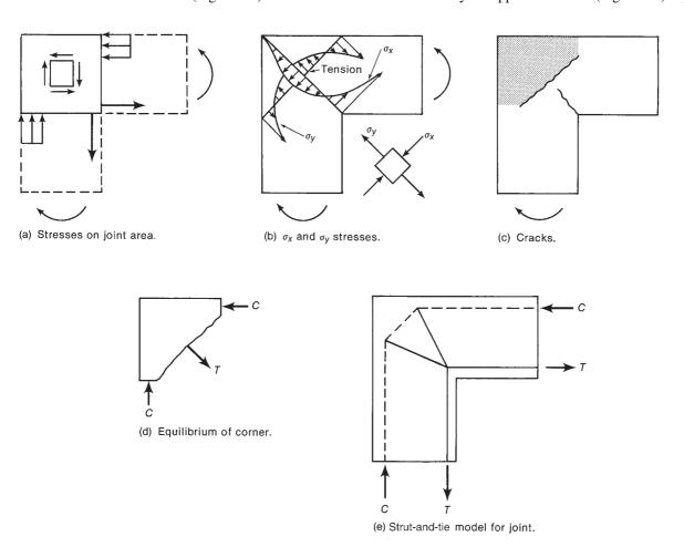
Fig. 17-45 Stresses in an opening joint.
