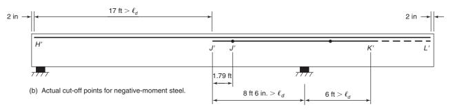
Fig. 8-33 Location of negative-moment cut-off points—Example 8-5.
