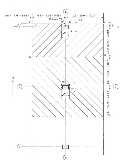
Fig. 13-87 Initial critical shear perimeters and tributary areas for columns *B*1 and *B*2.
