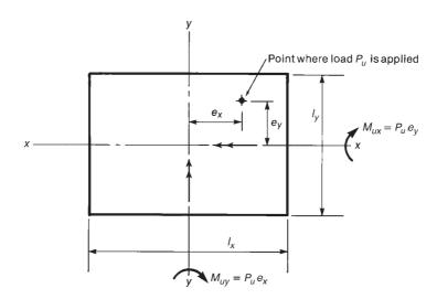
Fig. 11-33 Definition of terms: biaxially loaded columns.
