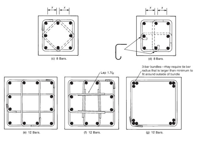
Fig. 11-29 Typical tie arrangements.
