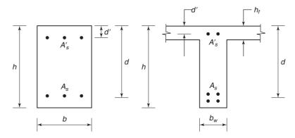
Fig. 4-6 Typical doubly reinforced sections in positive bending.
