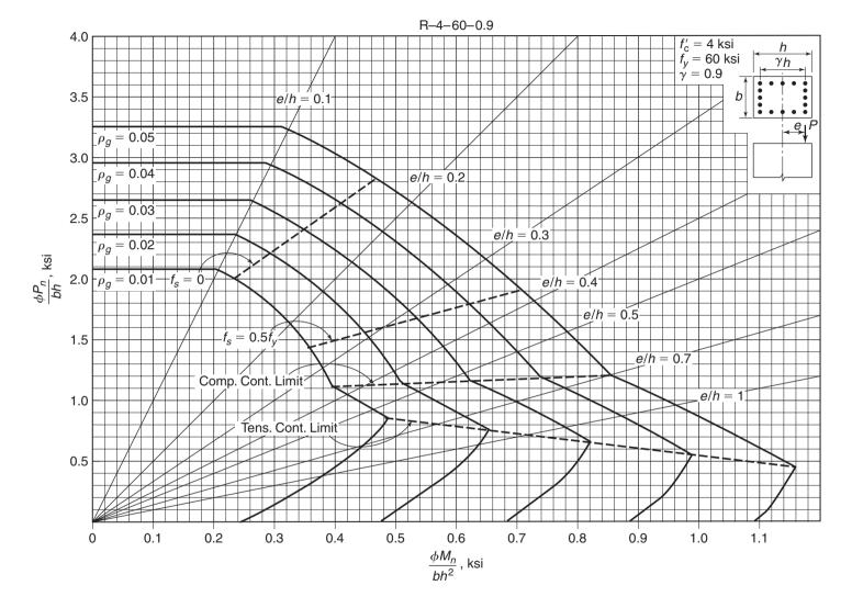
Fig. A-9c Nondimensional interaction diagram for rectangular tied column with bars in four faces:  $f'_c = 4000$  psi and  $\gamma = 0.90$ .
