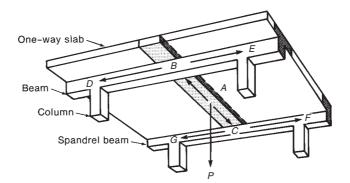
Fig. 4-1 One-way flexure.
