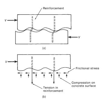
Fig. 16-4 Shear-friction model. (From [16-6].)
