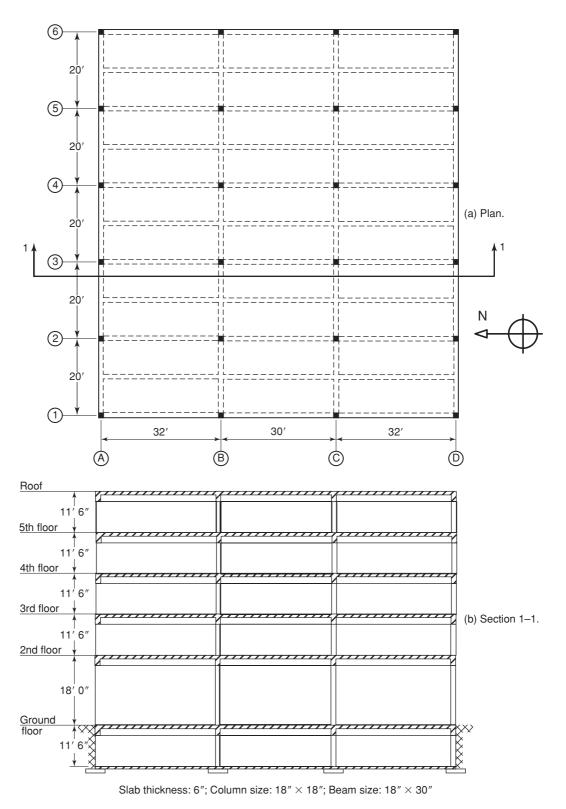
Fig. 12-32 Plan and elevation of sway frame—Example 12-3.
