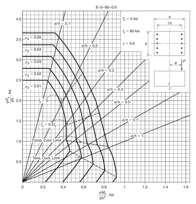
Fig. A-7a Nondimensional interaction diagram for rectangular tied column with bars in two faces:  $f_c' = 5000$  psi and  $\gamma = 0.60$ .
