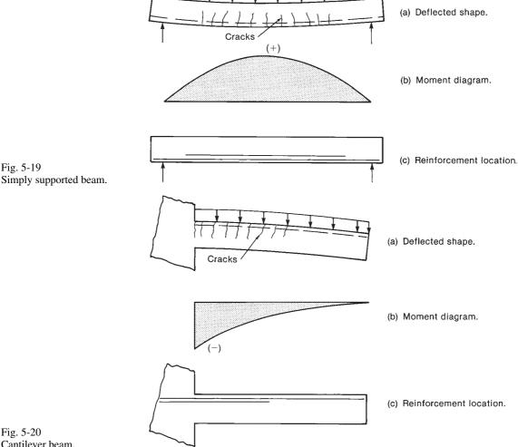
Fig. 5-20 Cantilever beam.
