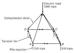
(b) Internal forces in pile cap.
