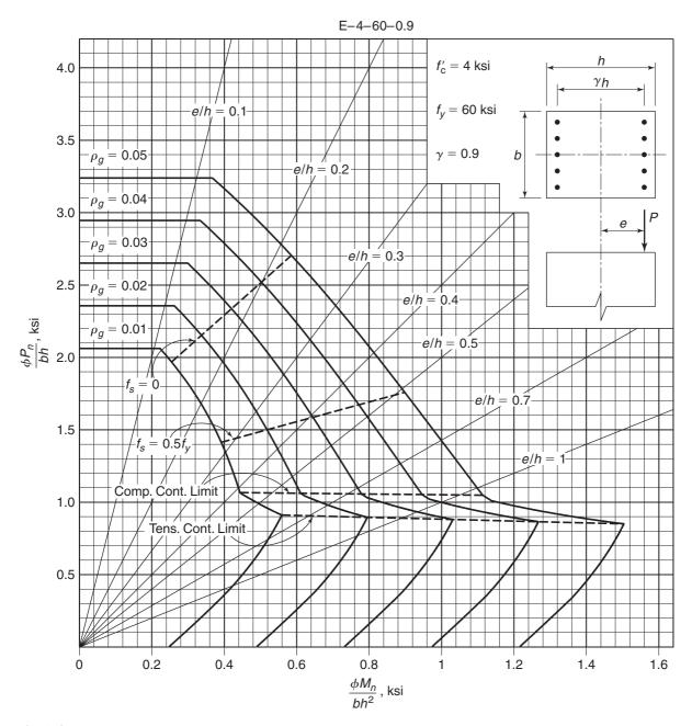
Fig. A-6c Nondimensional interaction diagram for rectangular tied column with bars in two faces:  $f'_c = 4000$  psi and  $\gamma = 0.90$ .
