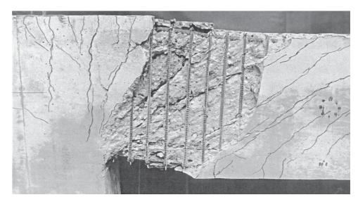
Fig. 6-22 Compression fan at interior support of the beam shown in Fig. 6-21b. (Photograph courtesy of J. G. MacGregor.)
