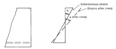
Fig. 9-15 Effect of creep on strains and curvature.
