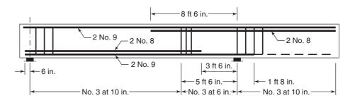
Fig. 8-34 Reinforcement details—Example 8-4.
