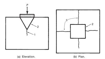
Fig. 17-58 Failure in a bearing test.
