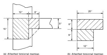
Fig. 13-30 Slab, column, and edge beam for Example 13-4.
