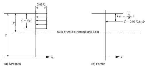
Fig. 4-16 Equivalent rectangular stress block.
