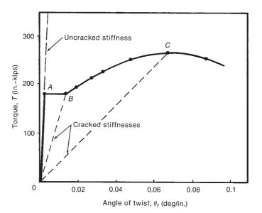
Fig. 7-12 Torque twist curve for a rectangular beam. (From [7-4].)
