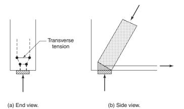
Fig. 17-6 Transverse spread of forces through the thickness of a strut.
