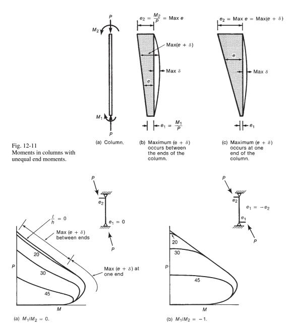
Fig. 12-12 Effect of  $M_1/M_2$  ratio on slender column interaction curves for hinged columns. (From [12-1].)
