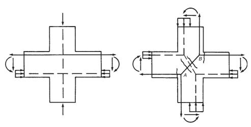
Fig. 17-52 Interior beam-column joint.
