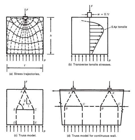
Fig. 17-57 Internal forces near bearing areas. (Adapted from [17-1].)
