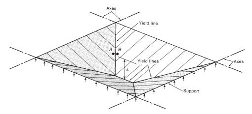
Fig. 14-4 Deformations of a slab with yield lines.
