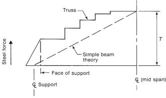
Fig. 17-13 Strut-and-tie model of a deep beam with dead load and stirrups.
