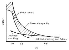
Fig. 6-8 Effect of *a/d* ratio on shear strength of beams without stirrups.
