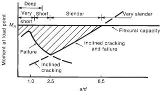
(b) Moments at cracking and failure.
