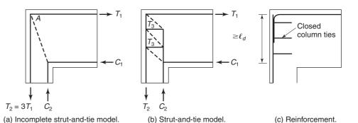
Fig. 17-48 Closing joint, beam deeper than column.
