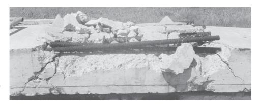
Fig. 8-38 Failure of a tension lap splice without stirrups enclosing the splice. (Photograph courtesy of J. G. MacGregor.)
