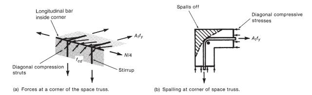
Fig. 7-25 Compressive strut forces at a corner of a torsional member.
