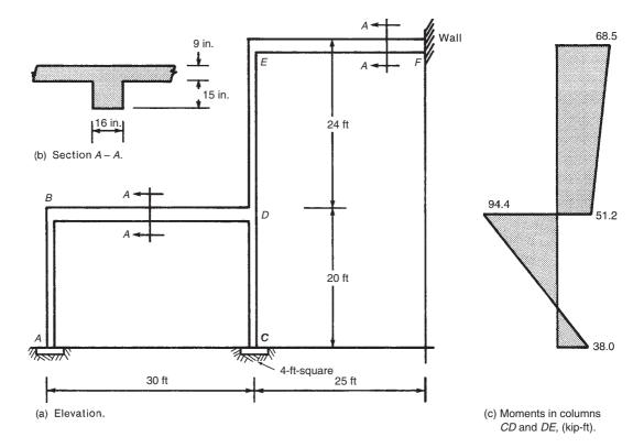
Fig. 12-28 Braced frame—Example 12-2.
