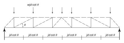
(c) Statically determinate truss.
