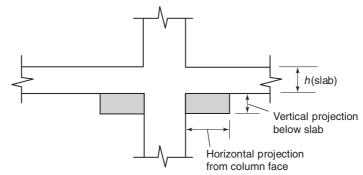
Fig. 13-82 Column capitals and shear caps for increased shear strength at slab-column connections.
