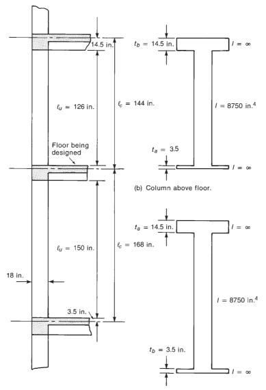
Fig. 13-42 Exterior columns to slab joint at *B*1 for Example 13-8.
