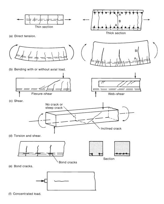
Fig. 9-3 Load-induced cracks. (From [9-5].)
