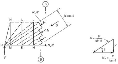
Fig. 6-24 Forces in stirrups and compression diagonals.
