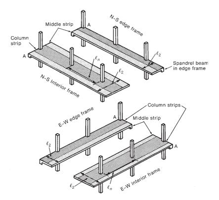
Fig. 13-20 Division of slab into frames for design.
