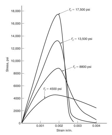
Fig. 3-18 Typical concrete stress–strain curves in compression. [Plotted using Eqs. (3-20) to (3-26).]
