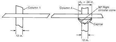
Fig. 13-21 Slab for Example 13-2.
