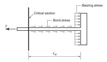
Fig. 8-15 Development length of headed bars in tension.
