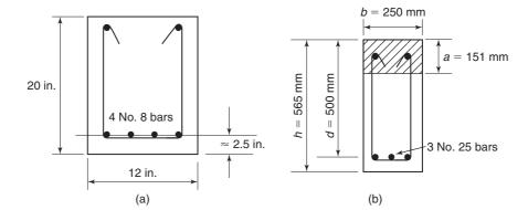
Fig. 4-19 Beam sections for (a) Example 4-1 and (b) Example 4-1M.
