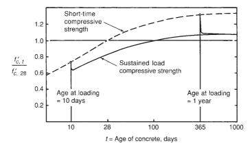
Fig. 3-2 Effect of sustained loads on the behavior of concrete in uniaxial compression. (From [3-4].)
