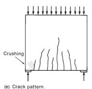
Fig. 17-27 Uniformly loaded deep beam. (Adapted from [17-1].)
