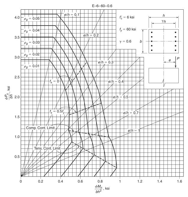
Fig. A-8a Nondimensional interaction diagram for rectangular tied column with bars in two faces:  $f_c' = 6000$  psi and  $\gamma = 0.60$ .
