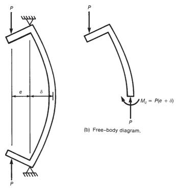
Fig. 12-1 Forces in a deflected column.
