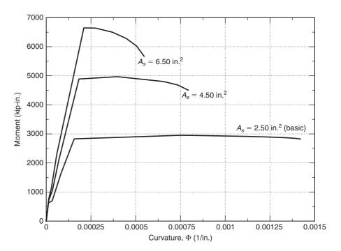
Fig. 4-11 Effect of increasing tension steel area,  $A_s$ .
