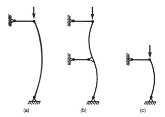
Fig. 12-5 Effective lengths of columns.
