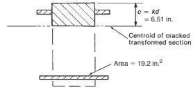
Fig. 9-1 Transformed sections— Example 9-1.
