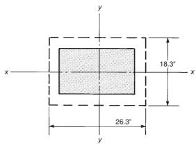
Fig. 13-91 Final critical shear perimeters for columns B1 and B2—Example 13-14.
