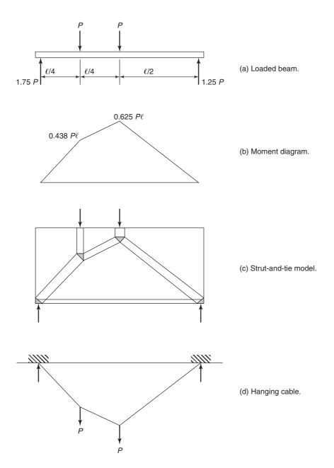
Fig. 17-22 Statical equivalence of various types of structures.
