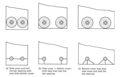
Fig. 8-8 Typical splitting-failure surfaces.
