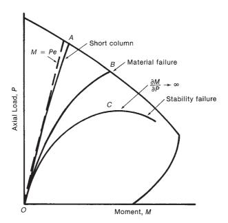
Fig. 12-8 Material and stability failures.
