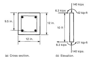
Fig. 6-46 Shear in column— Example 6-5.
