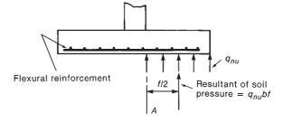
Fig. 15-7 Flexural action of a spread footing.
