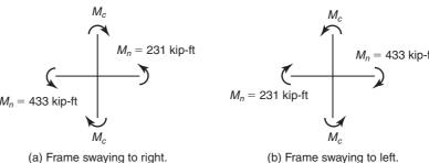
Fig. 19-26 Moments at a beam-column joint—Example 19-2.
