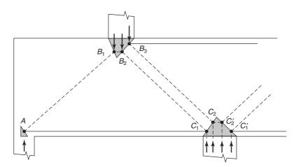
Fig. 17-32 Initial strut-and-tie model, two-span deep beam— Example 17-3.
