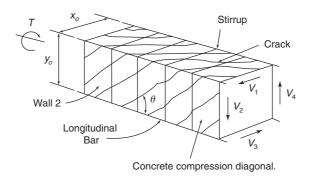
Fig. 7-15 Thin-walled tube analogy and space truss analogy.
