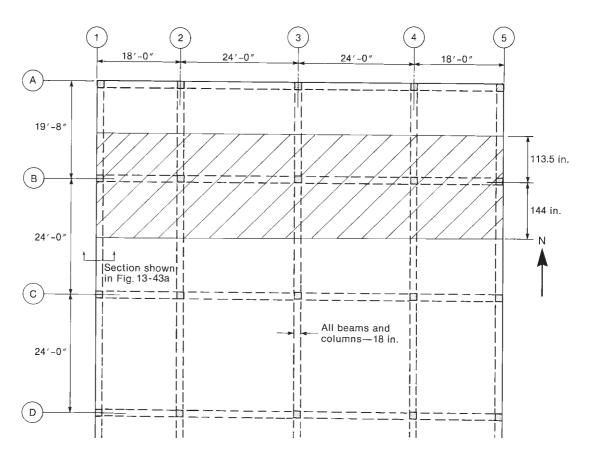
Fig. 13-35 Two-way slabs with beams—Examples 13-6 and 13-8.
