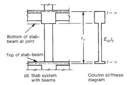
Fig. 13-37 Sections for the calculations of column stiffness,  $K_c$ .
