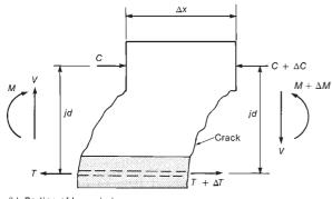
(b) Portion of beam between two cracks.
