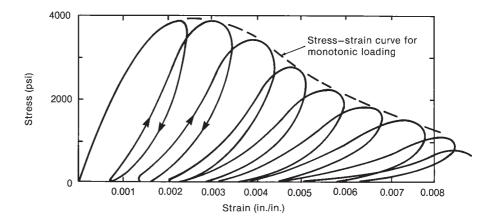
Fig. 3-20 Compressive stress–strain curves for cyclic loads. (From [3-45].)
