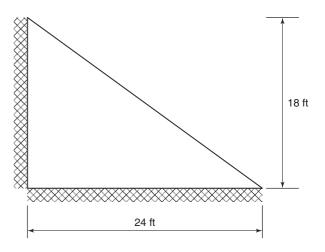
Fig. P14-4 Orthotropic positive reinforcement,  $m_{px} = 3$  k-ft/ft and  $m_{py} = 4$  k-ft/ft. and isotropic negative reinforcement with  $m_n = 5$  k-ft/ft.
