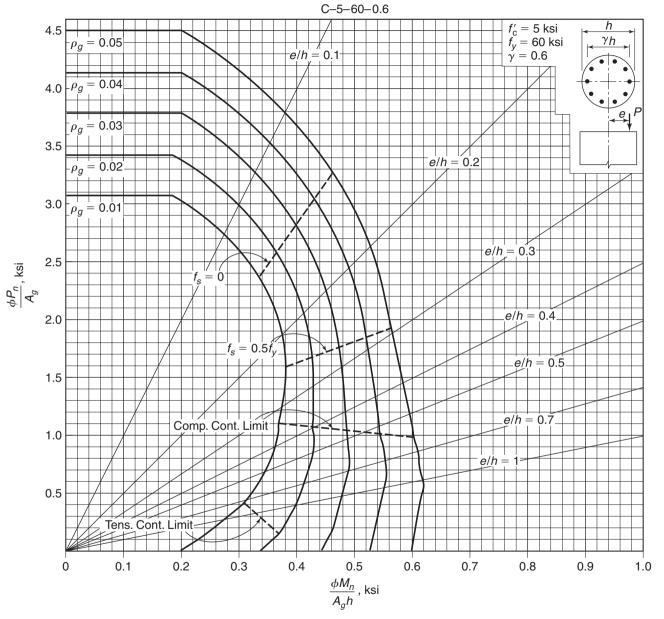
Fig. A-13a Nondimensional interaction diagram for circular spiral column:  $f_c' = 5000$  psi and  $\gamma = 0.60$ .
