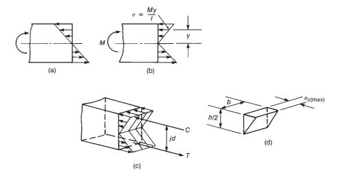
Fig. 4-4 Elastic beam stresses and stress blocks.
