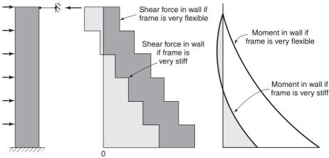
Fig. 18-7 Effect of frame stiffness on shear and moment in the shear wall.
