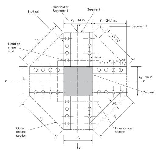
Fig. 13-70 Eight-sided critical shear section.
