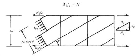
Fig. 7-18 Side of space truss—replacement of shear force  $V_2$ .
