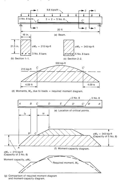
Fig. 8-19 Required moment and moment capacity.
