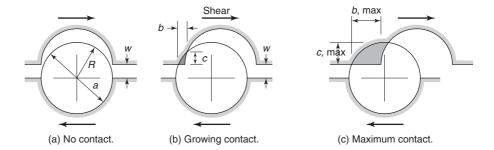
Fig. 16-8 Walraven crack model. (From [16-3].)
