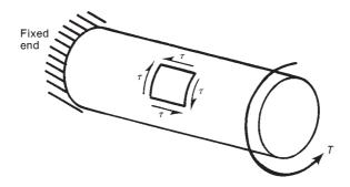
Fig. 7-1 Shear stresses due to torsion.
