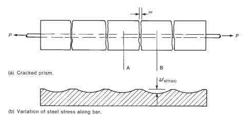
Fig. 9-7 Stresses in concrete and steel in a cracked prism.
