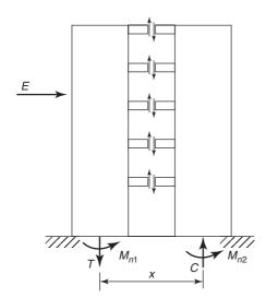
Fig. 19-34 Overturning moment resistance of coupled shear wall.
