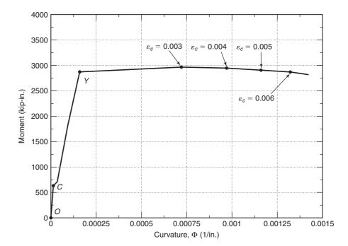
Fig. 4-10 Moment–curvature relationship for the section in Fig. 4.9(a) using  $f'_c = 4000$  psi and  $f_v = 60$  ksi.
