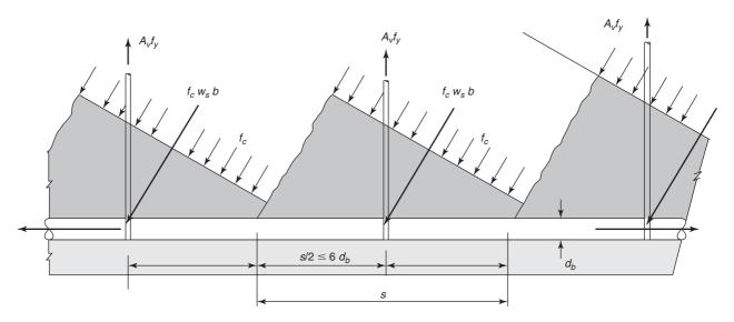
Fig. 17-16 Struts anchored by stirrups and longitudinal bars.
