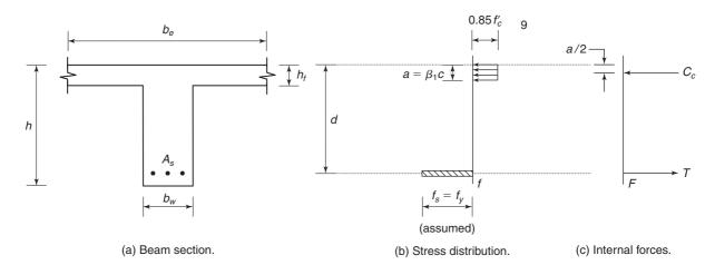
Fig. 4-43 Case 1 analysis  $(\beta_{1c} \le h_f)$  for  $M_n$  in T-section.
