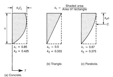
Fig. 4-15 Values of  $k_1$  and  $k_2$  for various stress distributions.
