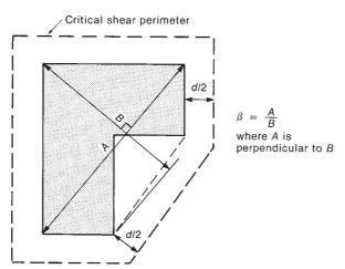
Fig. 13-60 Definition for irregular shaped columns.
