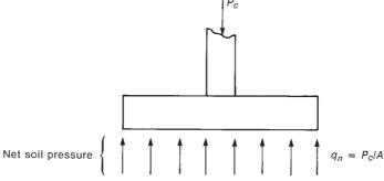
Fig. 15-6 Gross and net soil pressures.
