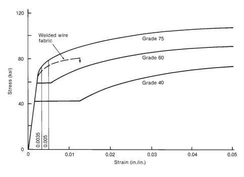
Fig. 3-31 Stress–strain curves for reinforcement.
