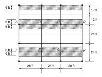
Fig. 5-4 Tributary areas for floor beams.
