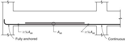
I structural-integrity rein(Must use at least two longitudinal bars at all locations)
