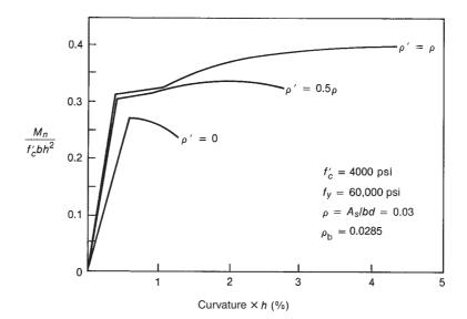
Fig. 4-32 Moment–curvature diagram for beams, with and without compression reinforcement. (From [4-16].)
