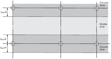
Fig. 13-23 Definitions of columns and middle strips.
