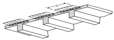
Fig. 4-40 Effective width of T-beams.
