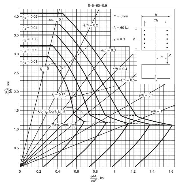
Fig. A-8c Nondimensional interaction diagram for rectangular tied column with bars in two faces:  $f'_c = 6000$  psi and  $\gamma = 0.90$ .
