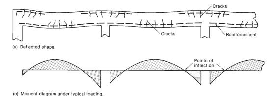
Fig. 8-18 Moments and reinforcement in a continuous beam.
