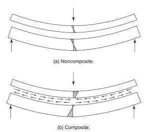
Fig. 16-11 Horizontal shear transfer in a composite beam.
