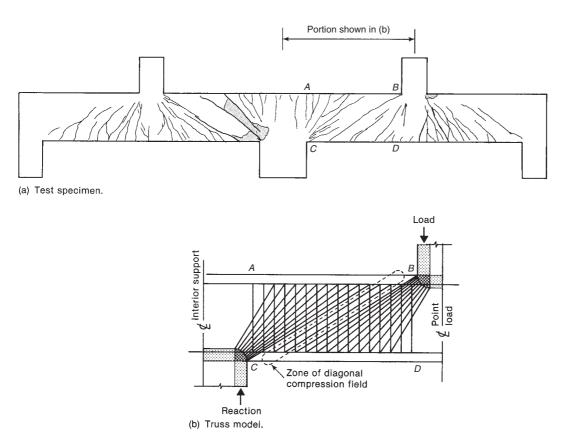
$Fig.\ 6\text{-}21$  Crack pattern and truss model for a two-span beam. (From [6-12].)
