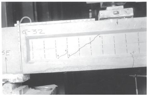
(a) Web-shear cracks.
