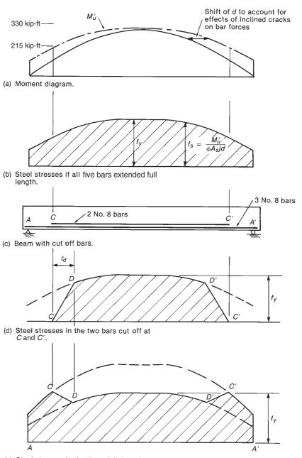
Fig. 8-21 Steel stresses in vicinity of bar cut-off points.
