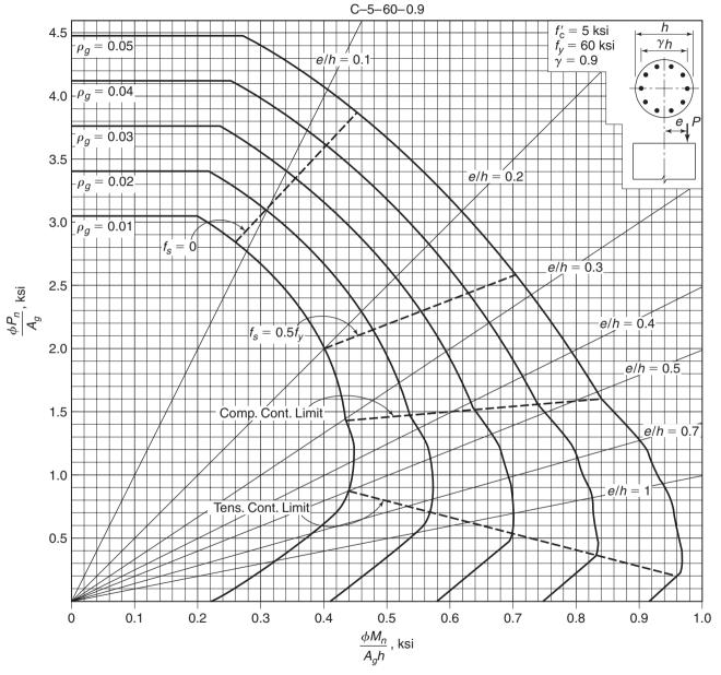
Fig. A-13c Nondimensional interaction diagram for circular spiral column:  $f'_c = 5000$  psi and  $\gamma = 0.90$ .
