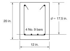
Fig. 4-27 Section used for Beams 1 and 2 of Example 4-3.
