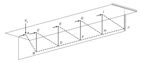
(a) Strut-and-tie model of beam web.
