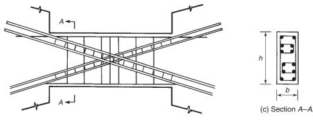
Fig. 19-35 Diagonally reinforced coupling beams.
