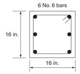
Fig. 12-17 Final column section for Example 12-1.
