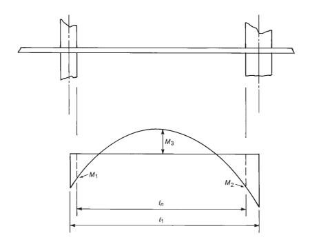
Fig. 13-45 Negative and positive moments in a slab beam.
