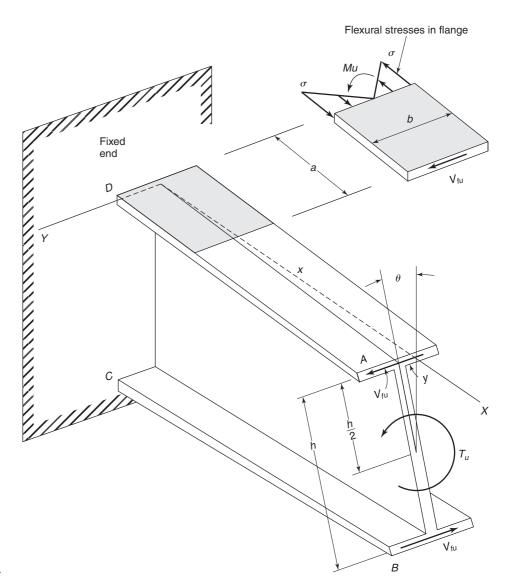
Fig. 7-10 Warping torsion of an I-beam.
