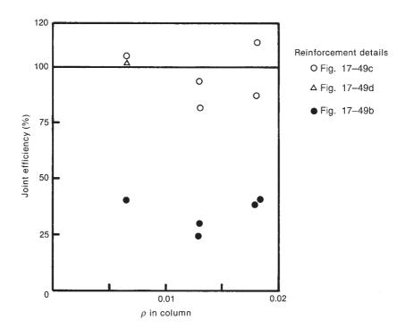
Fig. 17-50 Measured efficiency of T joints.
