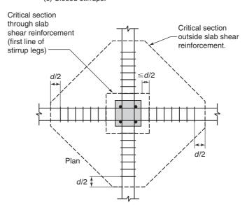
Fig. 13-66 Stirrup-type shear reinforcement in two-way slabs.
