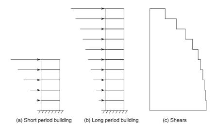
Fig. 19-12 Distribution of equivalent lateral forces and shears.
