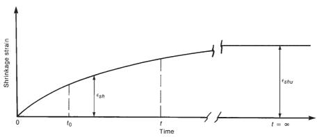
(a) Shrinkage of an unloaded specimen.
