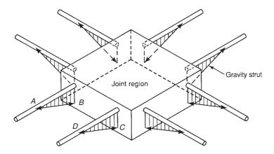
Fig. 13-54 Truss model for shear transfer at an interior column.
