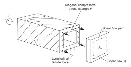
(a) Thin-walled tube analogy.
