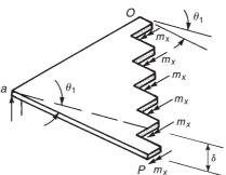
Rotation of slab Segment I about *y*-axis.
