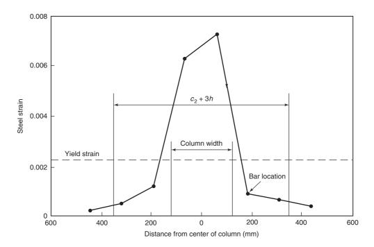
Fig. 13-74 Measured strains in bars adjacent to an edge column at failure. (From [13-41].)
