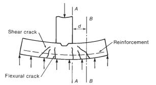
Fig. 15-11 Structural action of a strip footing.
