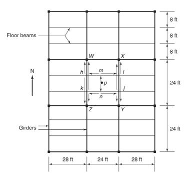
Fig. 5-2 Load paths in a one-way floor system.
