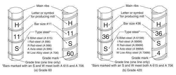
Fig. 3-30 Standard reinforcing-bar markings. (Courtesy of Concrete Reinforcing Steel Institute.)
