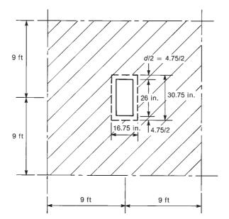
Fig. 13-64 Loaded area and critical sections for a two-way shear—Example 13-11.
