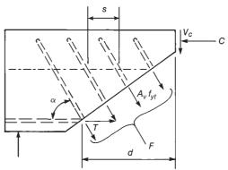
Fig. 6-26 Shear resisted by stirrups.
