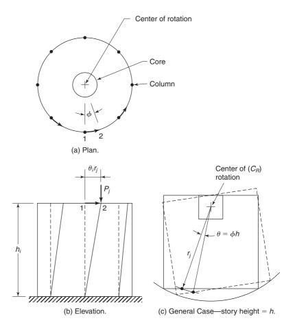
Fig. 12-36 Torsional critical load.
