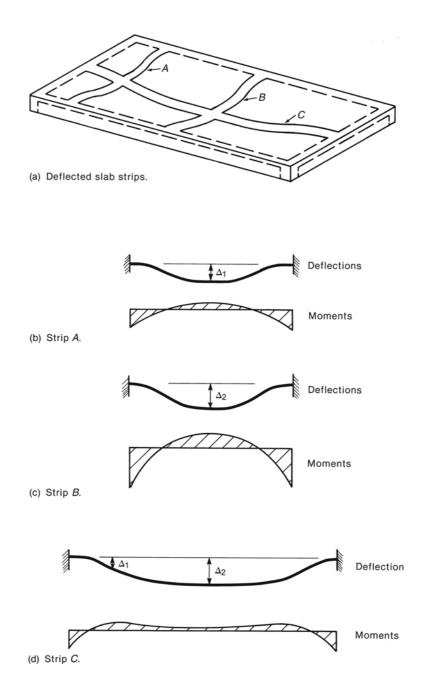
Fig. 13-9 Relationship between slab curvatures and moments.
