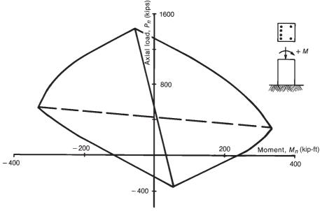
Fig. 11-21 Interaction diagrams for symmetrical and unsymmetrical columns.
