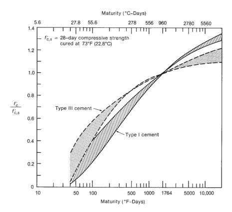
Fig. 3-8 Normalized compressive strength versus maturity. (From [3-23].)
