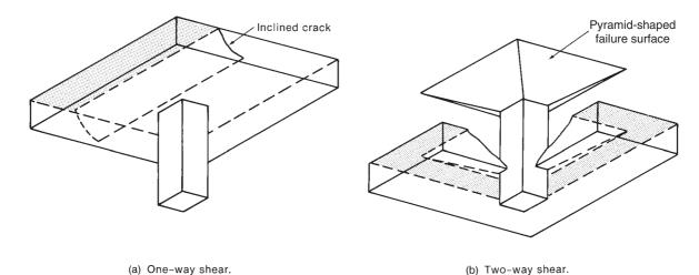
Fig. 13-52 Shear failure in a slab.
