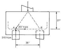
Fig. 15-25 Forces in a pile cap.
