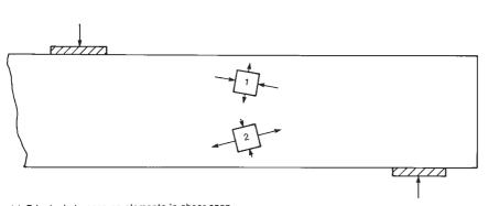
(c) Principal stresses on elements in shear span.
