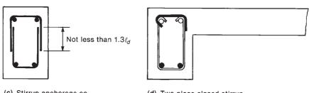
Fig. 6-30 Stirrup detailing requirements.
