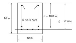
Fig. 4-28 Section used for Beam 3 of Example 4-3.
