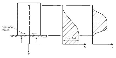
Fig. 8-6 Stress distribution in a pull-out test.
