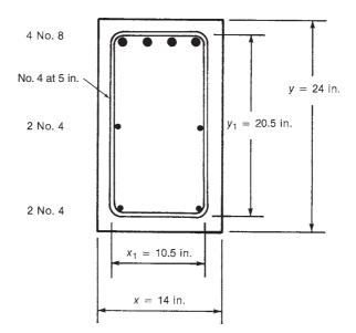
Fig. 7-29 Cross section of a cantilever beam—Example 7-2.
