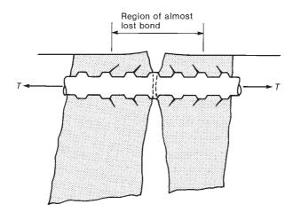
Fig. 9-8 Cracking at bar deformations. (From [9-2].)
