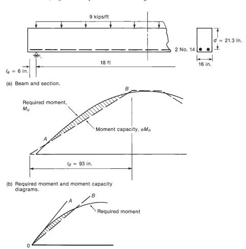
Fig. 8-22 Anchorage of positivemoment reinforcement.
