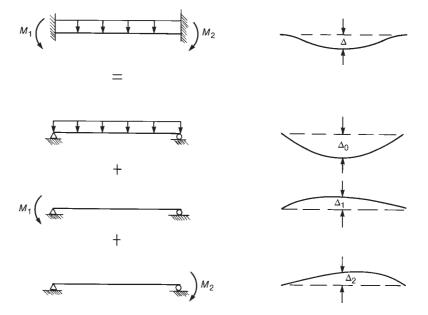
Fig. 9-14 Calculation of deflection for a beam with unequal end moments.
