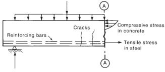
Fig. 1-4 Plain and reinforced concrete beams.
