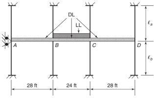
(b) Live load pattern to maximize positive moment at midspan of member *B*–*C*.
