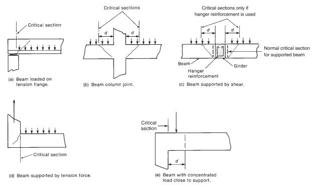
Fig. 6-33 Application of ACI Section 11.1.3.
