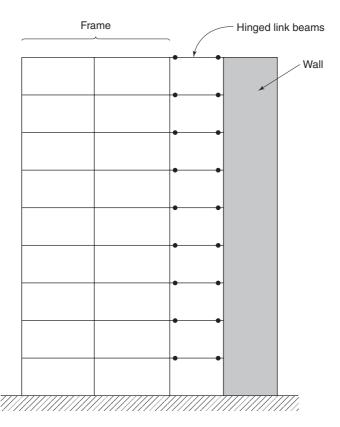
Fig. 18-6 Analytical model of a shear-wall–frame building.
