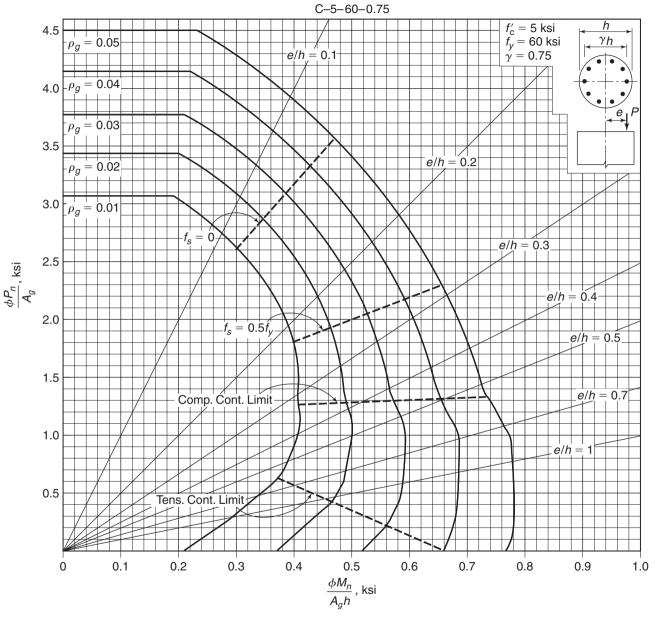
Fig. A-13b Nondimensional interaction diagram for circular spiral column:  $f'_c = 5000$  psi and  $\gamma = 0.75$ .
