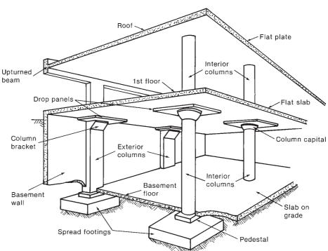
Fig. 1-7 Reinforced concrete building elements. (Adapted from [1-1].)
