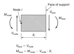
Fig. 5-15 Final design shear and moment at face of support.
