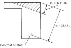
Fig. 4-51 Beam section for Example 4-7.
