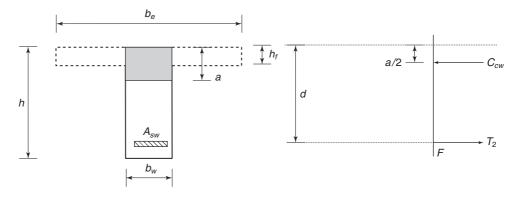
(c) Part 2: Web of section and corresponding internal forces.
