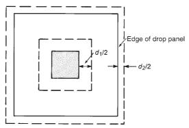
Fig. 13-56 Critical sections in a slab with drop panels.
