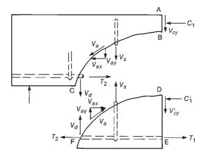
Fig. 6-17 Internal forces in a cracked beam with stirrups.
