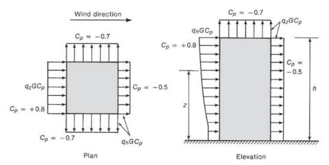
Fig. 2-11 Wind pressures and suctions on a building.
