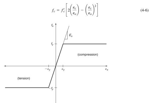
Fig. 4-7 Assumed stress–strain relationship for reinforcing steel.
