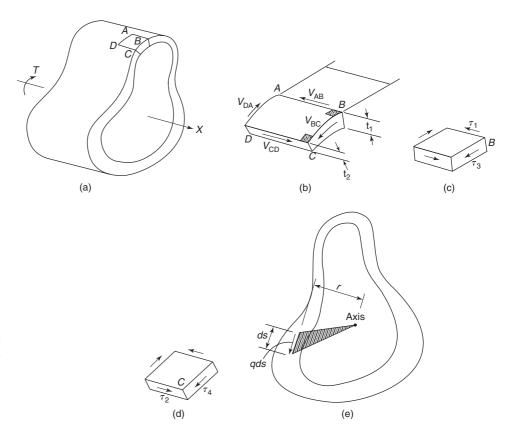
Fig. 7-6 Shear stresses in a thin-walled tube. (From [7-2] Popov, E. P., *Mechanics of Materials*, SI Version, 2/e © 1978, p. 80. Reprinted by permission of Prentice Hall, Upper Saddle River, New Jersey.)
