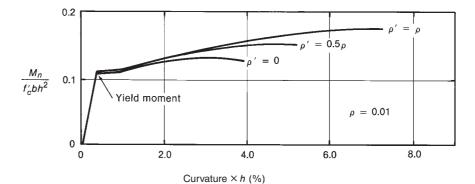
Fig. 4-31 Effect of compression reinforcement on strength and ductility of under-reinforced beams. (From [4-16].)
