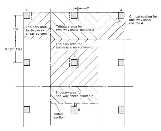
Fig. 13-58 Critical sections and tributary areas for shear in a flat plate.
