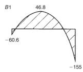
Fig. 13-98 Moments (kip-ft) in slab strips and beams on line B for Example 13-15.
