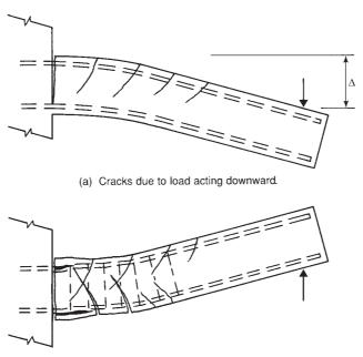
Fig. 19-13 Beam subjected to cyclic loads.
