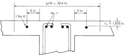
Fig. 10-8 Distribution of reinforcement.
