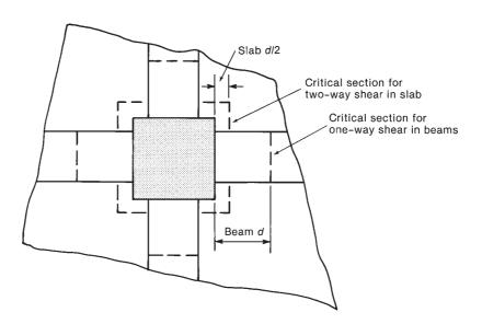
Fig. 13-94 Shear perimeters in slabs with beams.
