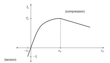
Fig. 4-8 Assumed stress–strain relationship for concrete.
