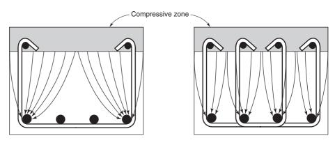
Fig. 6-28 Flow of diagonal compression force in the cross sections of beams with stirrups.
