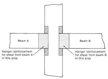
Fig. 6-41 Hanger reinforcement.
