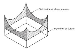
Fig. 13-59 Distribution of shear amount around the perimeter of a square.
