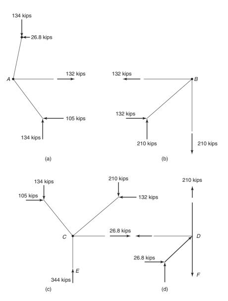
Fig. 17-40 Calculation of forces in struts and ties—Corbel— Example 17-4.
