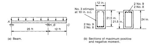
Fig. 8-29 Beam—Example 8-4.
