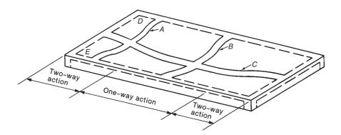
Fig. 10-13 One-way and two-way slab action near beam supports.
