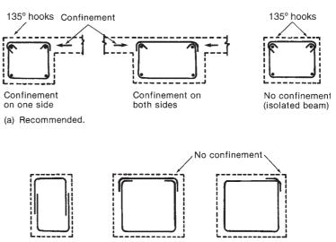
Fig. 7-26 Anchorage of closed stirrups. (From [7-12].)
