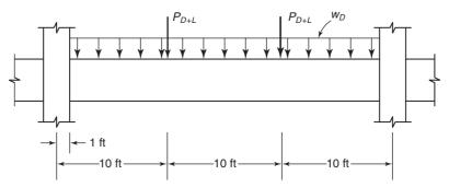
(a) Loads on girder for maximum shear at face of support.
