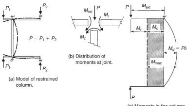
Fig. 12-18 Moments in a restrained column. (From [12-1].)
