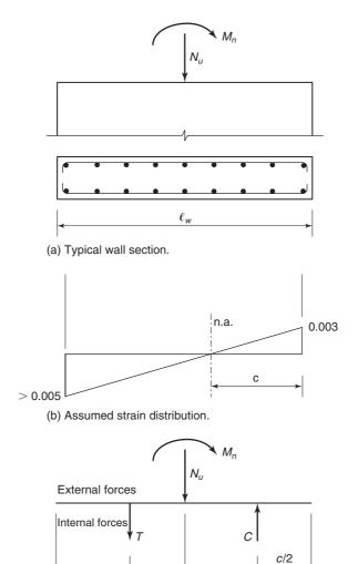
Fig. 18-15 Wall with uniform distribution of vertical reinforcement subjected to axial load and bending.
