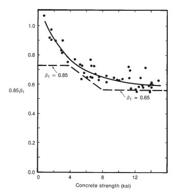
Fig. 4-17 Values of  $\beta_1$  from tests of concrete prisms. (From [4-7].)
