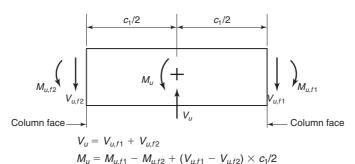
(c) Interior column, starting from moments and shears at column faces.
