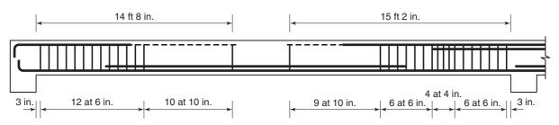
(a) Spacing of stirrups for beam B3.
