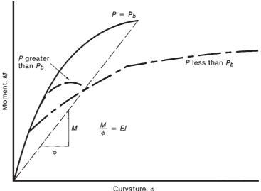
Fig. 12-14 Moment-curvature diagrams for a column cross section.
