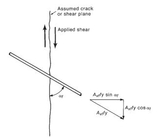
Fig. 16-5 Force components in a bar inclined to the shear plane. (From [16-1].)
