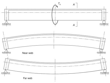
(a) Torsion acting on a double T-girder.
