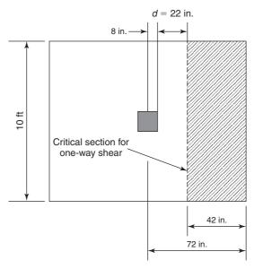
(a) Critical section for one-way shear.
