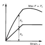
Fig. 11-8 Resistance of an axially loaded column.
