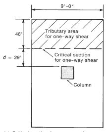
(a) Critical section for one-way shear.
