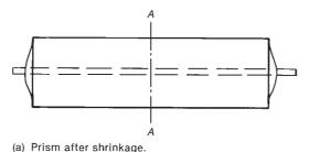
Fig. 2-8 Self-equilibrating stresses due to shrinkage.
