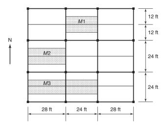
Fig. 5-9 Tributary areas for analysis and design of different beam sections.
