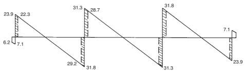
Fig. 13-47 Moments and shears in frame along line 2 for Example 13-9.
