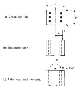
Fig. 11-9 Load and moment on column.
