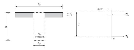
(b) Part 1: Overhanging flange(s) and corresponding internal forces.
