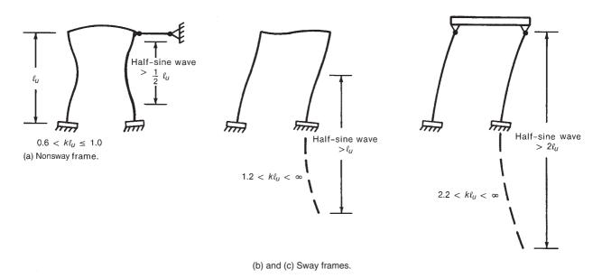
Fig. 12-25 Effective lengths of columns in frames with foundation rotations.
