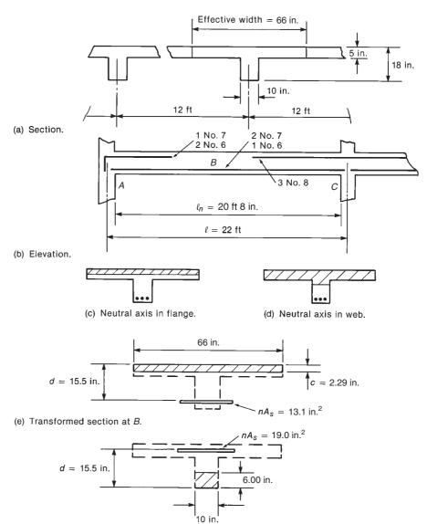
Fig. 9-17 End span of beam— Examples 9-5 and 9-6.
