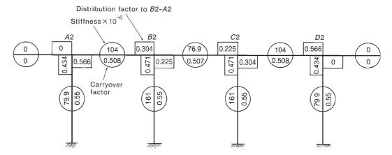
Fig. 13-46 Stiffness, carryover, and distribution factors—Example 13-9.
