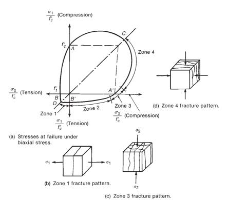
Fig. 3-12 Strength and modes of failure of unreinforced concrete subjected to biaxial stresses. (From [3-32].)
