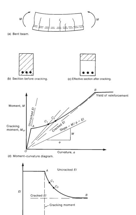
Fig. 9-11 Moment–curvature diagram and variation in *EI*.
