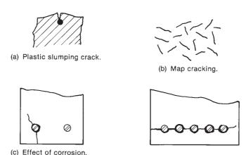
Fig. 9-5 Other types of cracks.
