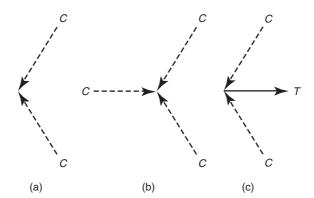
Fig. 17-9 Forces acting on nodes.
