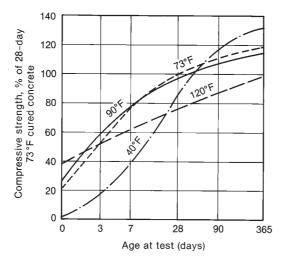
has proposed the following equation to represent the rate of strength gain for concrete made from Type I cement and moist-cured at 70°F:
