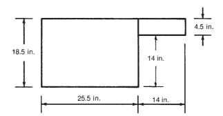
Fig. 7-33 Effective section for torsion— Example 7-4.
