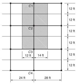
Fig. 5-30 Part of floor system used for design for Example 5-6.
