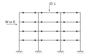
Fig. 13-51 Equivalent-frame model for analysis of slab—column frame subjected to gravity and lateral loads.
