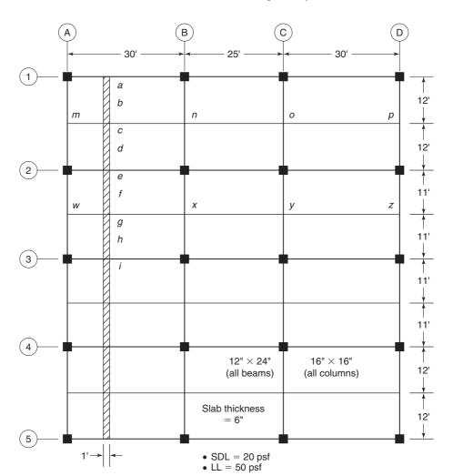
Fig. P7-3 Floor plan for Problems 7-3 and 7-4.
