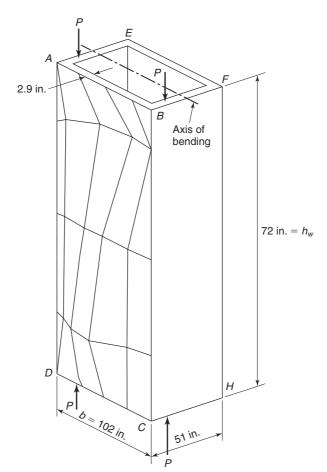
Fig. 18-26 Geometry, dimensions, and buckled shape of the compression flange of a hollow pier test specimen. (Note (a) that the concrete end blocks are not shown and (b) the deflections are plotted to an enlarged scaling). (From [18-21].
