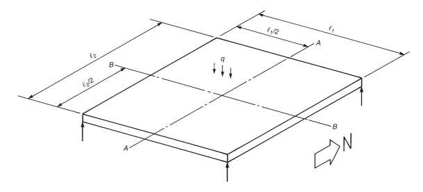
Fig. 13-7 Moments in a two-way slab.
