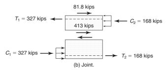
Fig. 19-29 Free-body diagrams of joint—Example 19-3.
