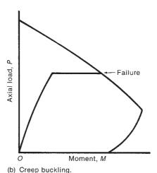
Fig. 12-15 Load-moment behavior for hinged columns subjected to sustained loads.
