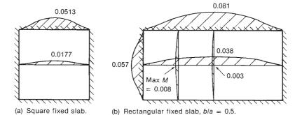
Fig. 13-14 Bending moments per unit inch in rectangular slabs with fixed edges. (From [13-4].)
