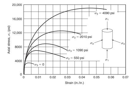
Fig. 3-15 Axial stress–strain curves from triaxial compression tests on concrete cylinders; unconfined compressive strength  $f'_c = 3600$  psi. (From [3-3].)
