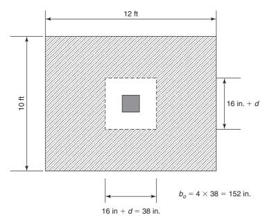
Fig. 15-17 Soil pressure distribution due to factored loads and critical shear perimeter.
