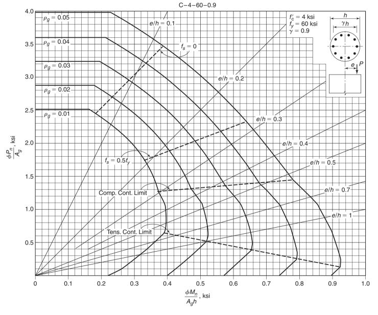
Fig. A-12c Nondimensional interaction diagram for circular spiral column:  $f'_c = 4000$  psi and  $\gamma = 0.90$ .
