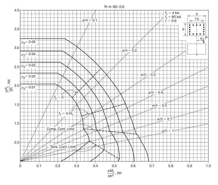
Fig. A-9a Nondimensional interaction diagram for rectangular tied column with bars in four faces:  $f'_c = 4000$  psi and  $\gamma = 0.60$ .
