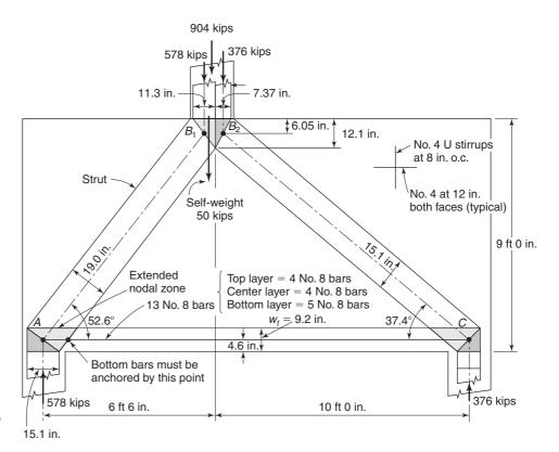
Fig. 17-31 Final design single-span deep beam—Example 17-2.
