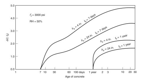
Fig. 3-25 Effect of effective thickness,  $h_e$ , and of age at loading,  $t_0$ , on creep coefficient.
