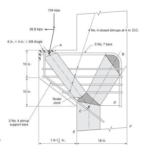
Fig. 17-38 Final strut-and-tie model of a corbel—Example 17-4.
