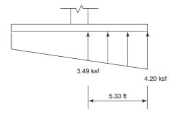
Fig. 15-18 Critical sections for one-way shear and bending.
