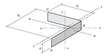
(c) Critical shear perimeter of corner column.
