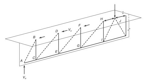
(a) Strut-and-tie model of beam web.
