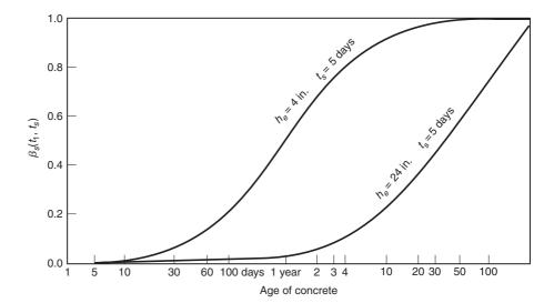
Fig. 3-24 Effect of effective thickness,  $h_e$ , on the rate of development of shrinkage.
