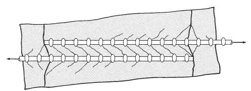
(b) Internal cracks at splice.
