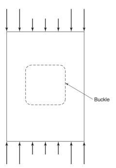
Fig. 18-25 Stresses in a plate after buckling.
