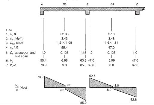
(a) Exterior end of B3. Because this beam is supported by other beams, the critical section for shear is located at the face of the support. ACI Code Section 11.4.6.1 requires stirrups if  $V_u \ge \phi V_c/2$ , where
