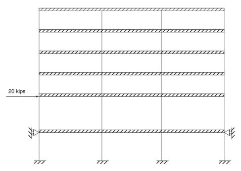
(a) Gravity load plus arbitrary lateral load to evalutate stability index, Q.
