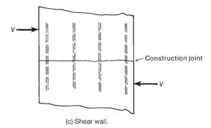
Fig. 16-7 Examples of shear friction. (From [16-9].)
