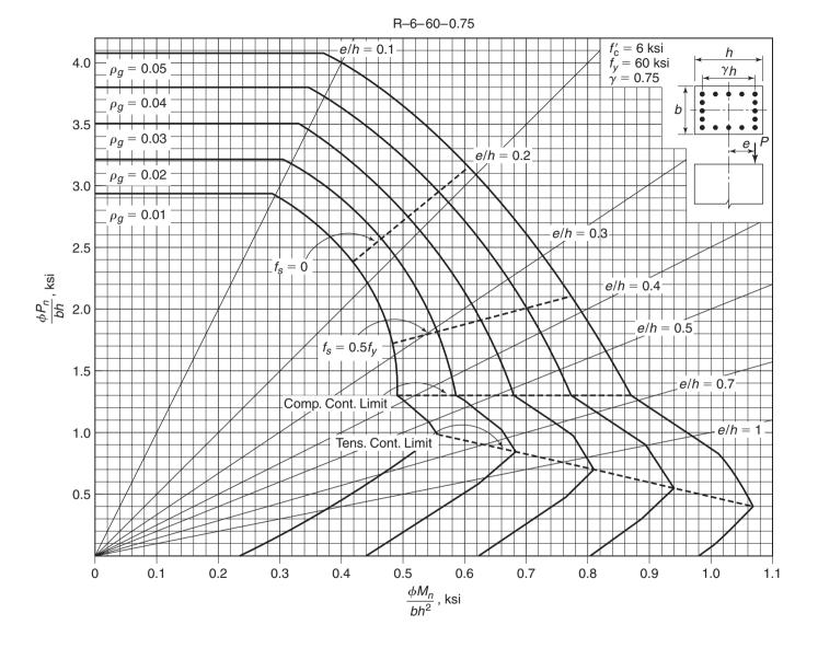
Fig. A-11b Nondimensional interaction diagram for tied column with bars in four faces:  $f'_c = 6000$  psi and  $\gamma = 0.75$ .
