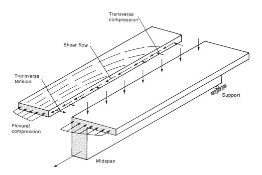
Fig. 4-39 Actual flow of forces on a T-beam flange.
