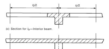
Fig. 13-17 Beam and slab sections for calculations of  $\alpha_f$ .
