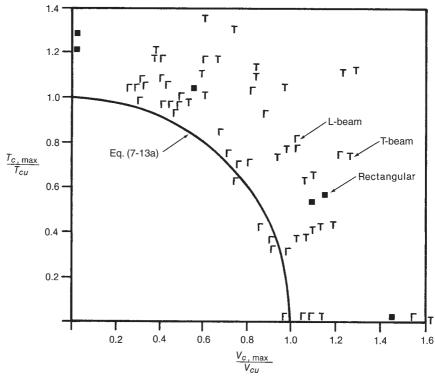
Fig. 7-14 Interaction of torsion and shear. (From [7-5].)
