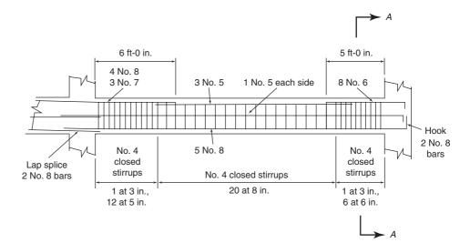
Fig. 7-36 Reinforcement in edge beam—Example 7-4.
