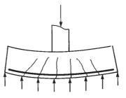
Fig. 15-20 Structural action of combined footing.
