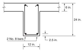
(b) Section design at midspan of beam A-B.
