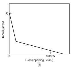
Fig. 3-21 Stress–strain curve and stress–crack opening curves for concrete loaded in tension.
