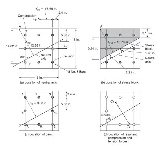
Fig. 11-35 Location of neutral axis and stress block—Example 11-5.
