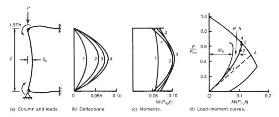
Fig. 12-20 Behavior of a short restrained column bent in symmetrical single curvature.  $\ell/h = 15$ ,  $k\ell_u/r = 33$ ,  $\rho_g = 0.01$ ,  $K_b = 2.5K_c$  at both ends. (From [12-16].)
