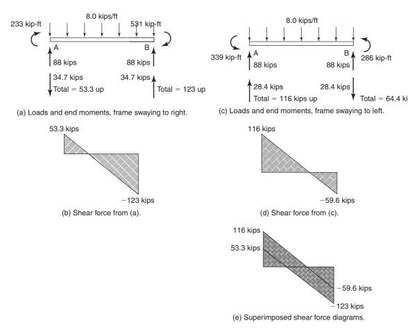
Fig. 19-21 Computation of shear forces—Example 19-1.
