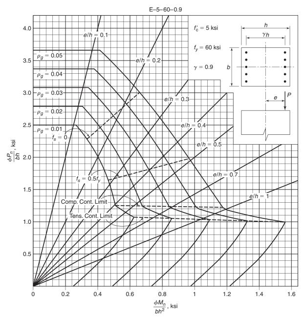
Fig. A-7c Nondimensional interaction diagram for rectangular tied column with bars in two faces:  $f'_c = 5000$  psi and  $\gamma = 0.90$ .
