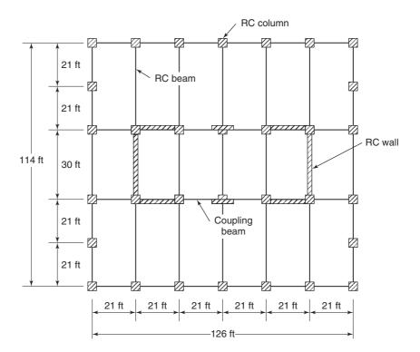
Fig. 18-12 General building floor plan.
