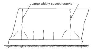
Fig. 9-4 Heat-of-hydration cracking.
