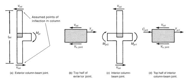
Fig. 17-53 Calculation of shear in joints.
