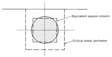
Fig. 13-78 Critical shear perimeters for moments and shear transfer at circular columns.
