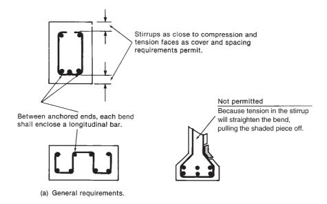
Standard stirrup hook, ACI Section 7.1.3, Must enclose a bar, ACI Section 12.13.2.1
