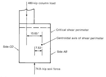
Fig. 15-22 Shear calculations at exterior column—Example 15-5.
