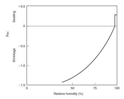
Fig. 3-23 Effect of relative humidity on shrinkage.
