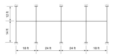
Fig. 13-97 Frame used for the analysis of the two-way slab in Example 13-15.
