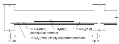
(a) Beams that are not part of primary lateral load-resisting system.
