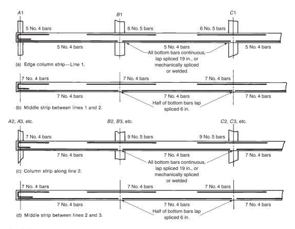
Fig. 13-89 Schematic diagram of reinforcement in east—west strips for Example 13-14.
