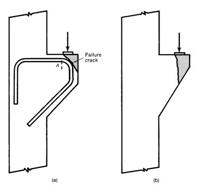
Fig. 17-39 Failure of corbels due to poor detailing.
