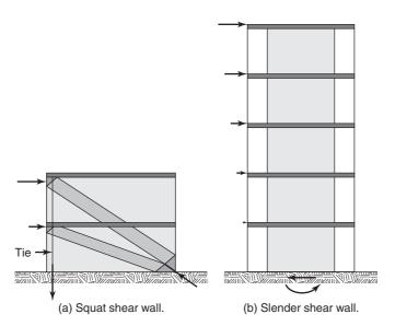
Fig. 18-4 Shear walls.
