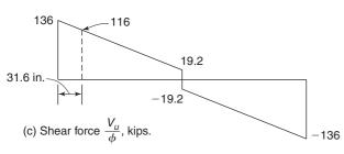
Fig. 6-37 Beam and shear force envelope—Example 6-2.
