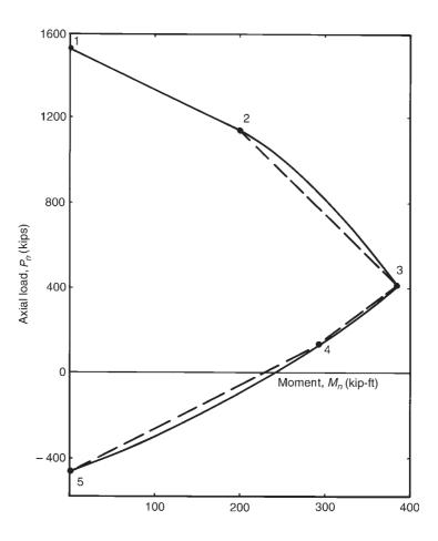
Fig. 11-22 Simplified interaction diagram.
