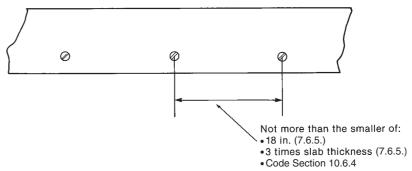
Fig. 5-23 Bar spacing limits in ACI Code.
