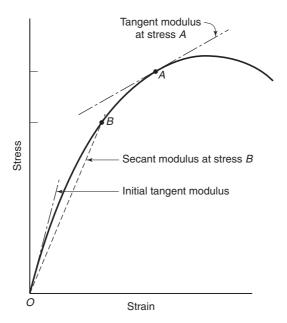
Fig. 3-17 Tangent and secant moduli of elasticity.
