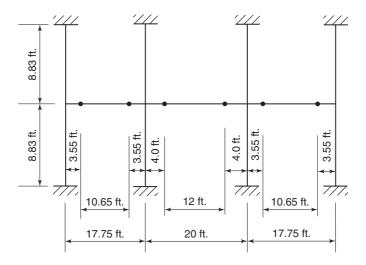
Fig. 13-50 Dimensions and node point locations for slab-column frame analyzed in Example 13-10.
