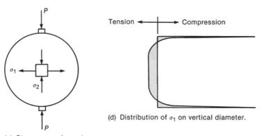
Fig. 3-9 Split-cylinder test.
