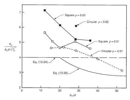
Fig. 13-61 Comparison of design equations to test data.
