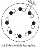
A shall not be less than  $1\frac{1}{2}$  in.,  $1\frac{1}{2}$  bar diameters or  $1\frac{1}{3}$  times aggregate size.
