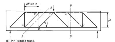
Fig. 6-19 Truss analogy.
