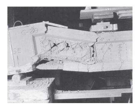
Fig. 6-25 Web crushing failure. (Photograph courtesy of J. G. MacGregor.)
