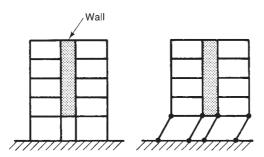
Fig. 19-8 Soft story due to discontinued shear walls.
