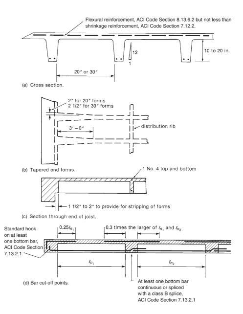
Fig. 10-15 One-way-joist construction.
