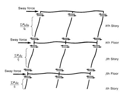
Fig. 12-31 Iterative  $P-\Delta$  analyses.
