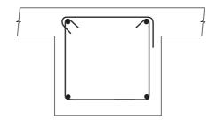
Fig. 19-22 No. 4 two-leg closed hoop— Example 19-1.
