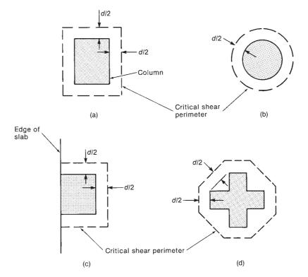
Fig. 13-55 Location of critical shear perimeters.
