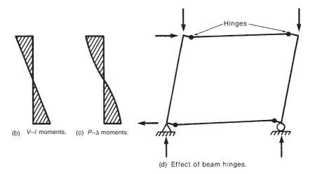
Fig. 12-30 Column moments in a sway frame.
