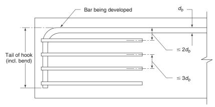
Fig. 8-14 Confinement of hooks by stirrups and ties.
