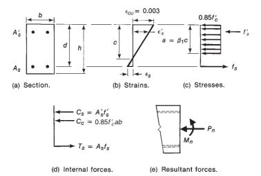
Fig. 11-12 Calculation of  $P_n$  and  $M_n$  for a given strain distribution.
