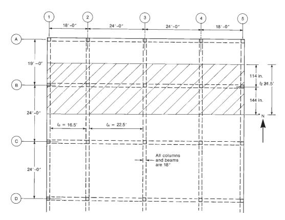
Fig. 13-95 Plan of a two-way slab with beams for Example 13-15.
