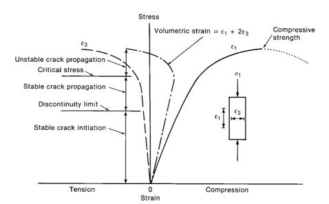
Fig. 3-1 Stress-strain curves for concrete loaded in uniaxial compression. (From [3-2].)
