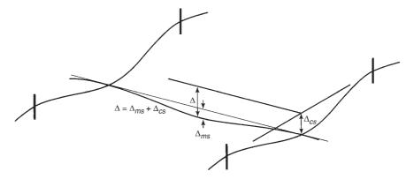
Fig. 13-100 Superposition of column strip and middle strip deflections.
