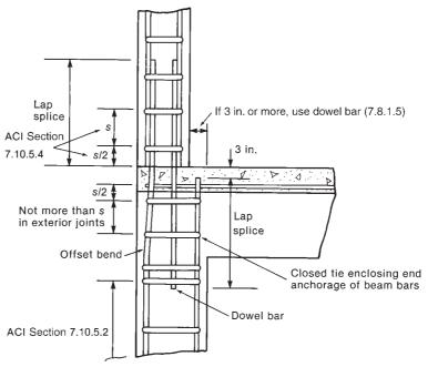
Fig. 11-25 Lap Details at column–beam joints following given ACI Code Sections.
