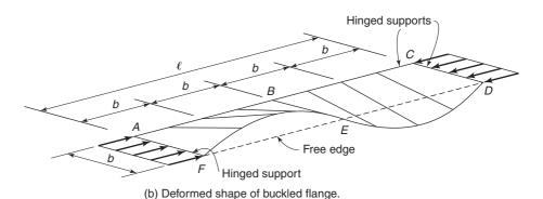
Fig. 18-27 Buckling of an outstanding flange of a wall assemblage.
