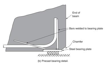
Fig. 8-23 Simple beam supports.
