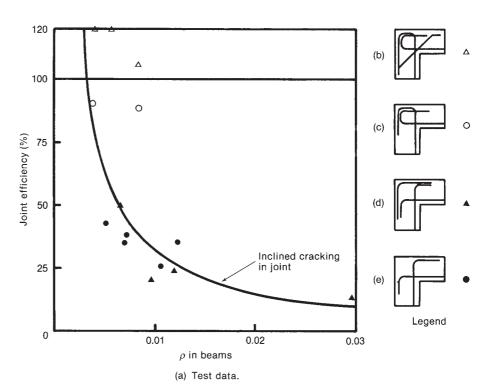
Fig. 17-46 Measured efficiency of opening joints.
