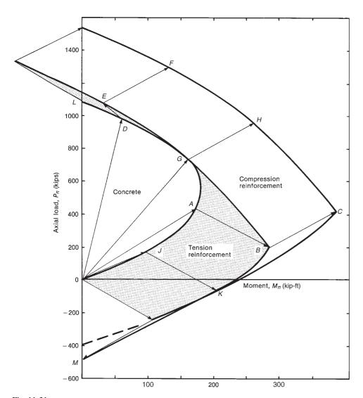
Fig. 11-31 Components of interaction diagram—Example 11-1.
