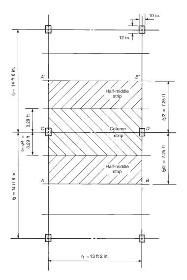
Fig. 13-25 Interior panel of a flat plate for Example 13-3.
