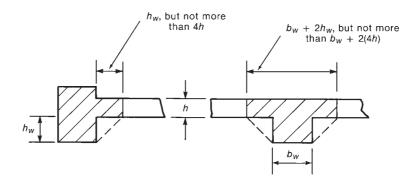
Fig. 13-18 Cross section of beams as defined in ACI Code Section 13.2.4.
