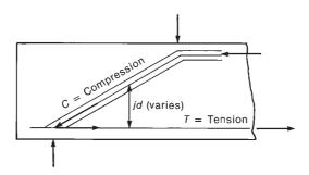
Fig. 6-6 Arch action in a beam.
