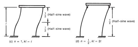
Fig. 12-6 Effective lengths of idealized columns.
