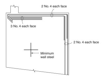
Fig. 17-20 Reinforcement in the wall in Fig. 17-19.
