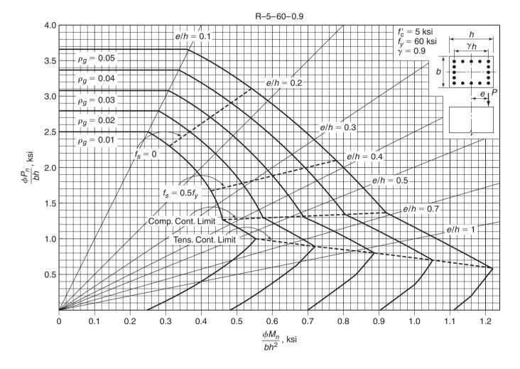
Fig. A-10c Nondimensional interaction diagram for tied column with bars in four faces:  $f'_c = 5000$  psi and  $\gamma = 0.90$ .
