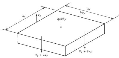
Fig. 14-1 Moments and forces in a medium-thick plate.
