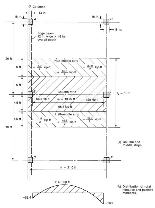
Fig. 13-28 Calculation of moments in an end span—Example 13-4.
