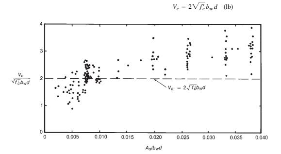
Fig. 6-14 Effect of reinforcement ratio,  $\rho_w$ , on shear capacity,  $V_c$ , of beams constructed with normal-weight concrete and without stirrups. [6-7]
