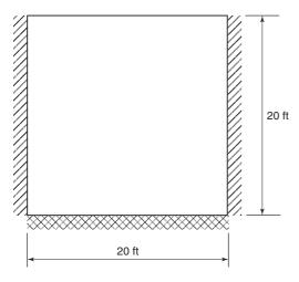
Fig. P14-2 Isotropic reinforcement,  $m_n = 8 \text{ k-ft/ft}$  and  $m_p = 4.5 \text{ k-ft/ft}$ .
