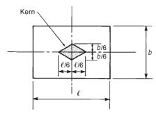
Soil pressure under a footing: loads within kern.
