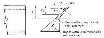
Fig. 4-29 Effect of compression reinforcement on moment strength.
