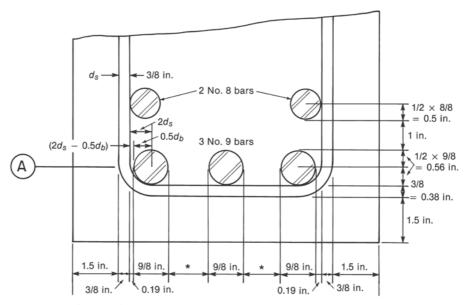
Fig. 5-25 Beam section for Example 5-3.
