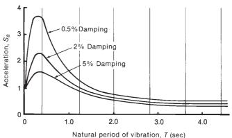
Fig. 19-1 Earthquake response spectrum.
