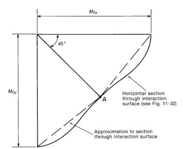
Fig. 11-34 Approximation of section through intersection surface.
