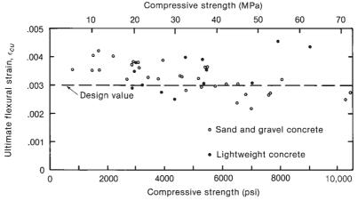
Fig. 4-13 Limiting compressive strain. (From [4-6] and [4-7].)
