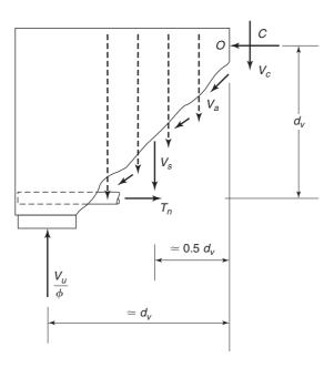
Fig. 6-31 Free-body diagram of beam reaction zone.
