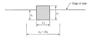
Fig. 13-84 Width effective for moment transfer at exterior columns.
