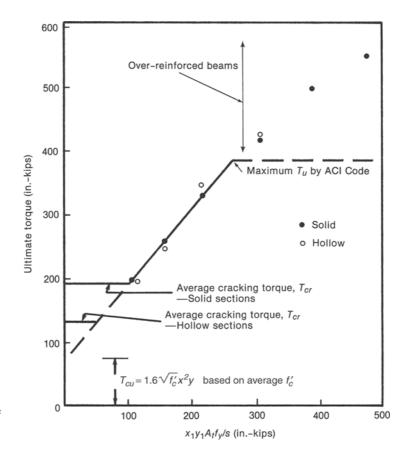
Fig. 7-13 Torsional strength of solid and hollow sections with the same outside dimensions. (From [7-4].)
