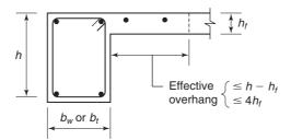
Fig. 7-16 Part of overhanging flange effective for torsion.
