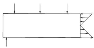
(a) Stresses acting on a cross section.
