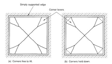
Fig. 14-14 Corner levers in simply supported slabs.
