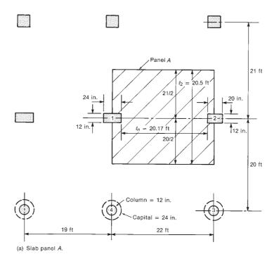
Fig. 13-21 Slab for Example 13-2.
