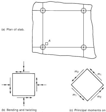
Fig. 14-15 Principal moments adjacent to a column in a flat plane.
