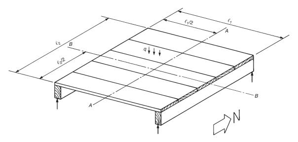
Fig. 13-6 Moments in a plank-and-beam floor.
