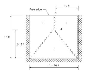
Fig. 14-12 Slab panel and plastic mechanism for Example 14-6.
