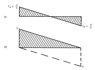
Fig. 7-23 Torques in beam *A*–*B* of the structure shown in Fig. 7-21c.
