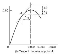
Fig. 18-24 Second-order parabolic stress–strain curve for compressed concrete.
