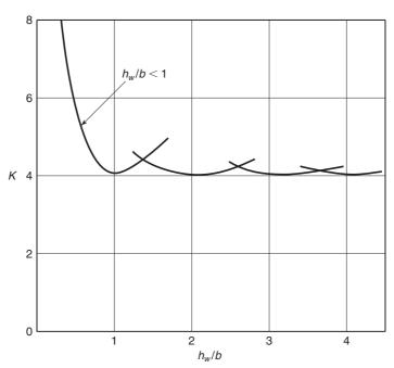
Fig. 18-23 Wall buckling factor, *K*, for buckling of a compressed plate analogous to a compressed wall in a hollow rectangular bridge pier. (From [18-4].)
