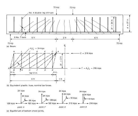
Fig. 6-20 Construction of an analogous plastic truss.
