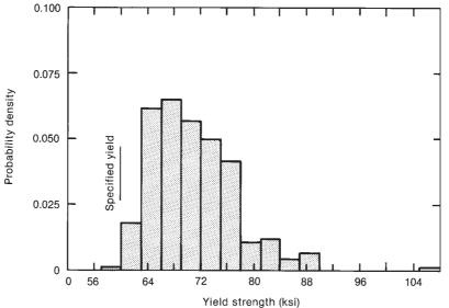
Fig. 3-32 Distribution of mill-test yield strengths for Grade-60 steel. (From [3-72].)
