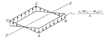
(c) Shear due to unbalanced moment.
