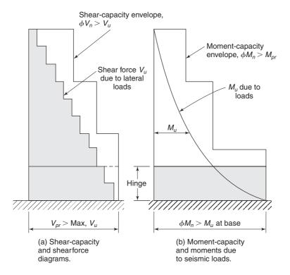
Fig. 19-15 Capacity design of a shear wall.
