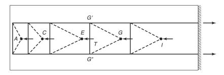
Fig. 17-60 Strut-and-tie models of a T beam with the flange in tension.
