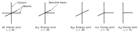
Fig. 17-54 Classification of joints—ACI 352. ( $\gamma$  values are for Type-1 joints.)
