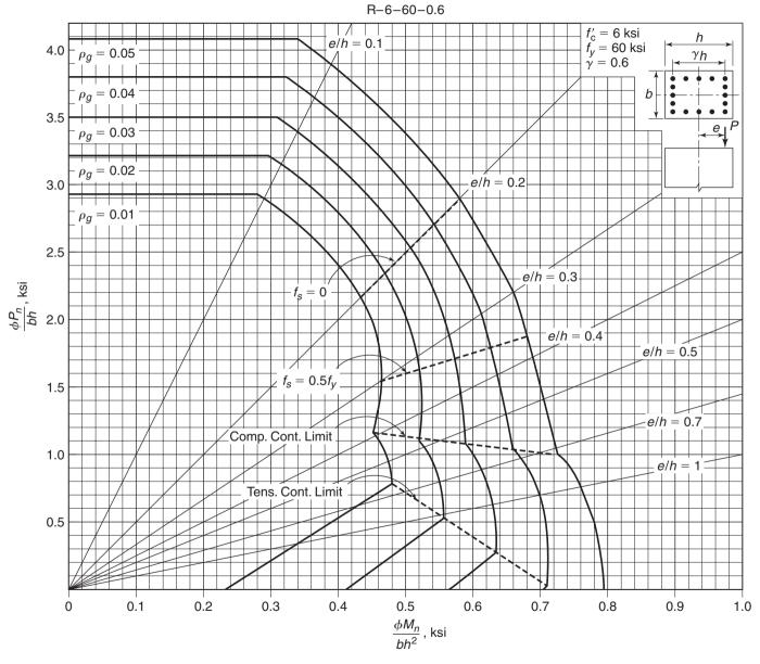
Fig. A-11a Nondimensional interaction diagram for tied column with bars in four faces:  $f'_c = 6000$  psi and  $\gamma = 0.60$ .
