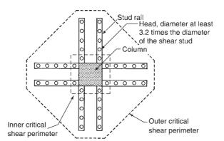
Fig. 13-68 Headed shear studs.
