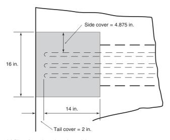
(a) Plan of exterior column-beam joint.
