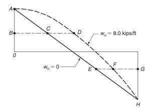
Fig. 19-23 Effect of uniform load on cut-off points.
