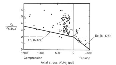
Fig. 6-16 Effect of axial loads on inclined cracking shear. From [6-7].
