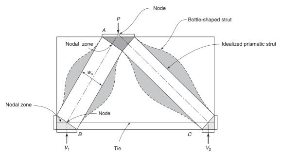
Fig. 17-3 Strut-and-tie model of a deep beam.
