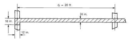
(a) Section through edge of slab.
