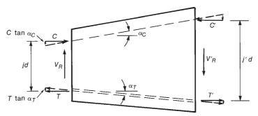
Fig. 6-43 Reduced shear force in nonprismatic beam.
