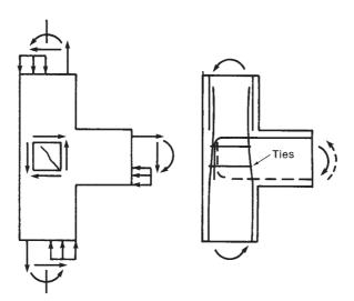
Fig. 17-51 Exterior beam-column joint.
