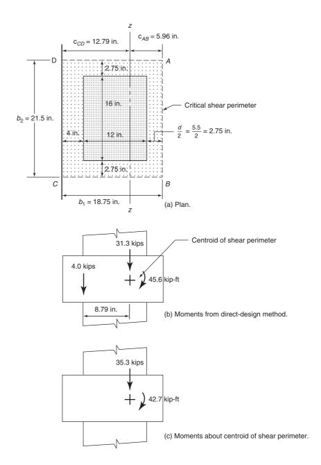
Fig. 13-80 Slab-column joint for Example 13-13.
