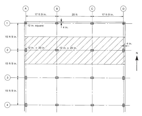
Fig. 13-34 Plan of a flat-plate floor—Examples 13-5, 13-7, 13-9, and 13-10.
