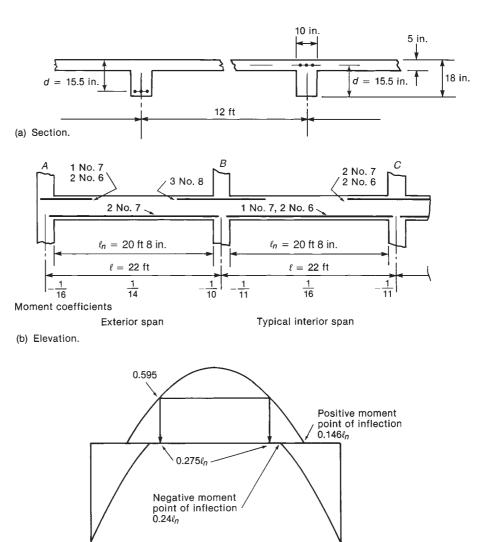
Fig. 8-35 Calculation of flexural cut-off points—Example 8-5.
