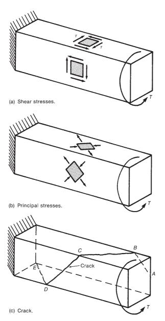
Fig. 7-8 Principal stresses and cracking due to pure torsion.
