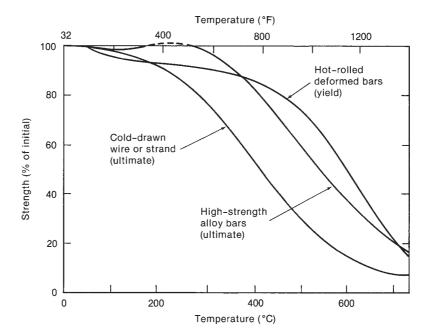
Fig. 3-34 Strength of reinforcing steels at high temperatures. (From [3-54].)
