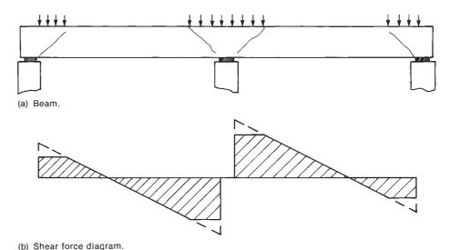
Fig. 6-32 Shear force diagram for design.
