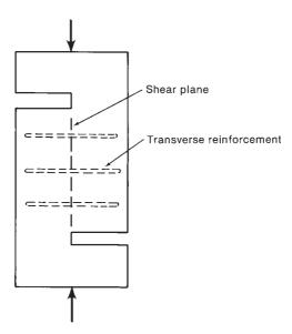
Fig. 16-1 Shear-transfer specimen.
