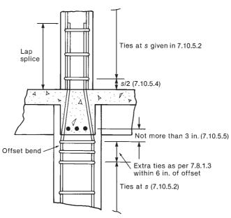
(a) Tie spacing at interior column-beam joint.
