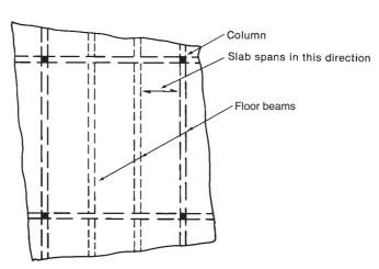
Fig. 5-1 Typical one-way floor systems.
