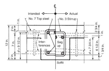
Fig. 5-24 Bar placing problems at the intersections of two beams. (From [5-4].)
