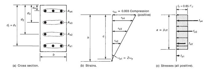
Fig. 11-14 Notation and sign convention for interaction diagram.
