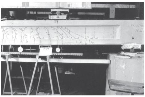
Fig. 6-12 Types of inclined cracks. (Photographs courtesy of J. G. MacGregor.)
