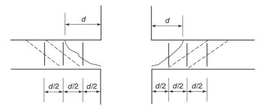
Fig. 13-69 Potential shear cracks and stirrup spacing at slab-column connection.
