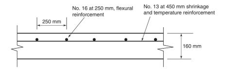
Fig. 5-38 Final slab section design for Example 5-7M.
