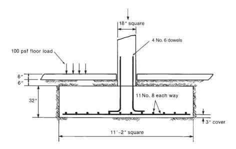
Fig. 15-13 Spread footing— Example 15-2.
