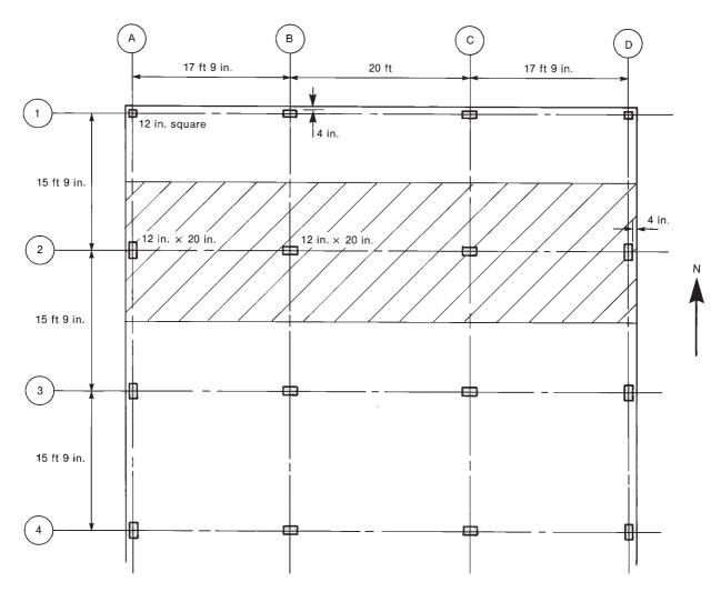
Fig. 13-85 Plan of flat-plate floor for Example 13-14.
