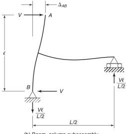
Fig. 18-5 Moment-resisting frame.
