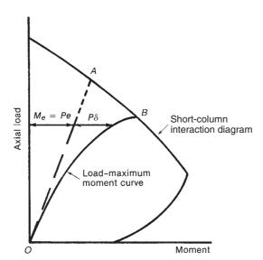
Fig. 12-2 Load and moment in a column.
