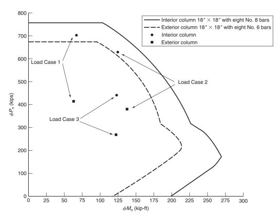
Fig. 12-35 Comparison of column strength and factored loads.
