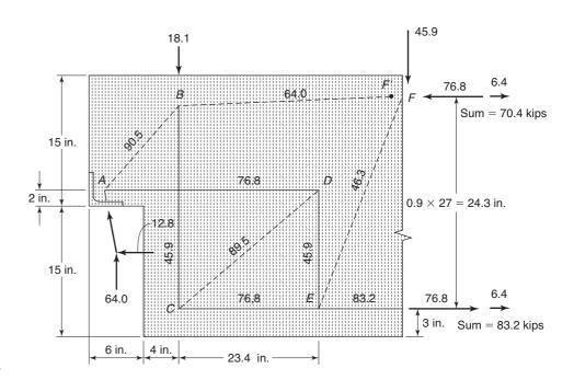
Fig. 17-43 Strut-and-tie model for a dapped end—Example 17-6.
