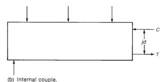
Fig. 2-2 Internal resisting moment.
